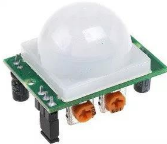
Figure 14: HC-SR501 PIR Sensor
