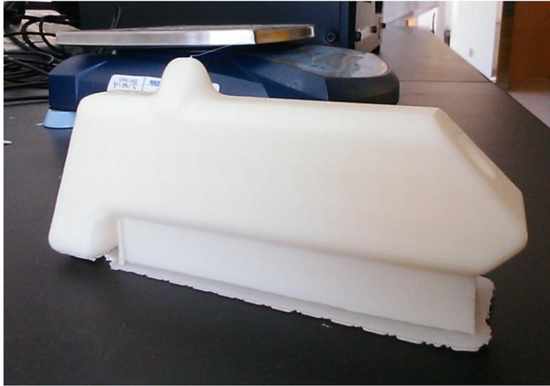
**Figure 22: Printed Shell of final ergonomic design**
