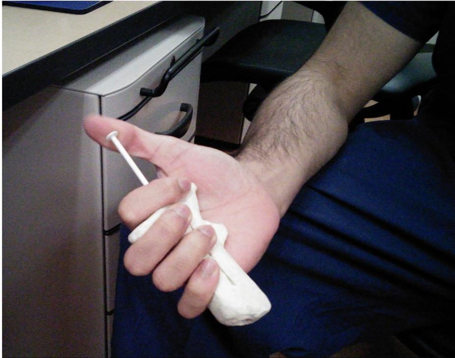
**Figure 17: Clay model testing of the ergonomics of the second iteration design**
