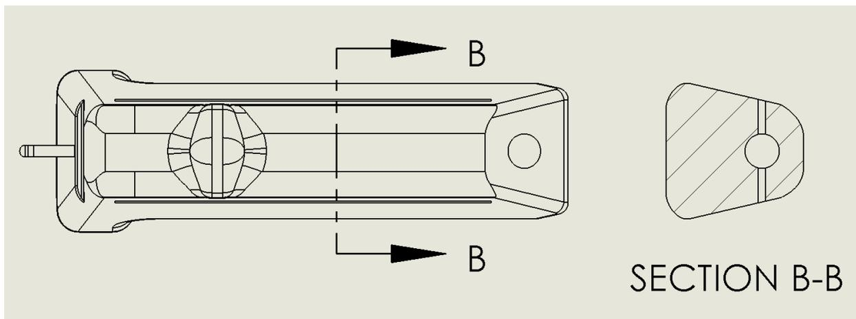
**Figure 19: Final design section view of ergonomic shell**
