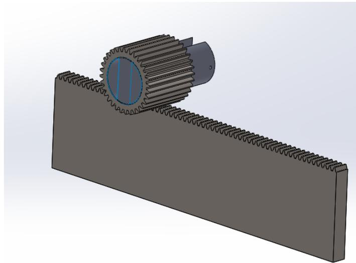
**Figure 7: Rack and Pinion CAD drawing**
