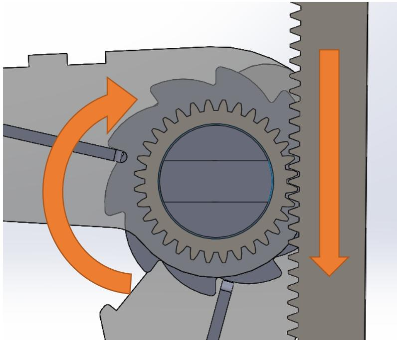
**Figure 21: Ratchet and rail combine to depress plunger**
