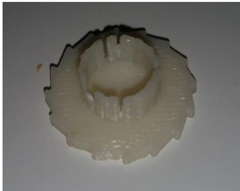
**Figure 24: Common printing defect at small scales**
