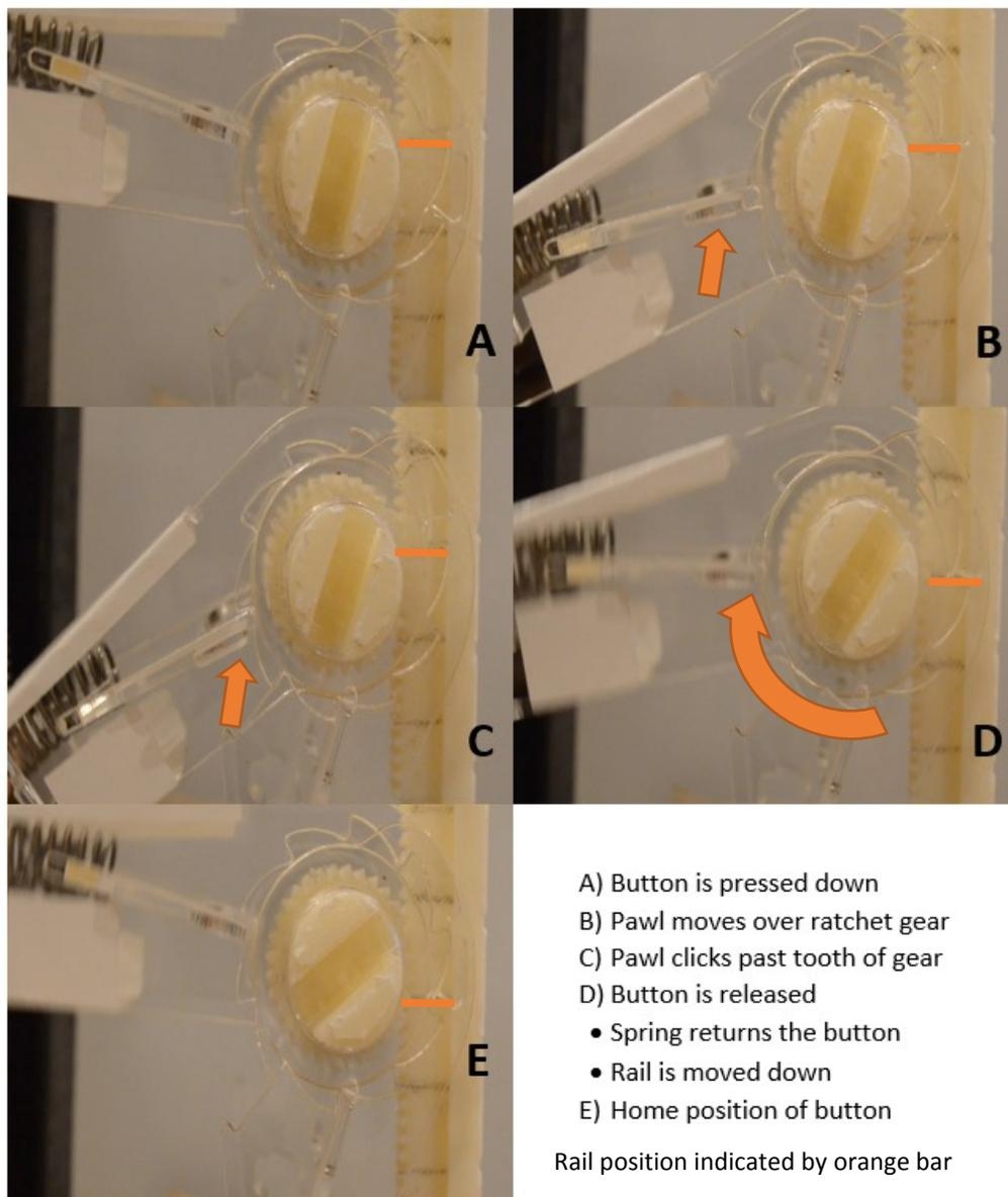
Figure 23: Proof of Concept Model showing the ratchet functionality of the deposition mechanism
