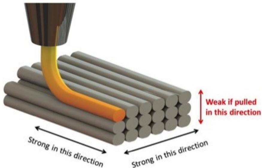
Figure 5: Fused deposition method (Ghose, 2015)
