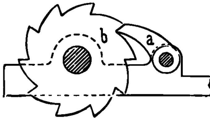
**Figure 6 Simple pawl (a) and ratchet (b) mechanism (Band, 1894)**
