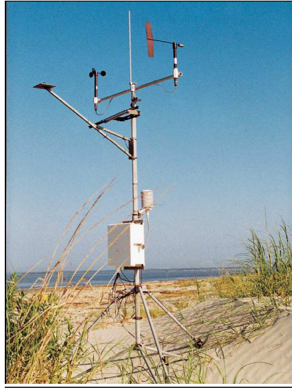
Figure 11: A CR1000 used in a weather station 10
