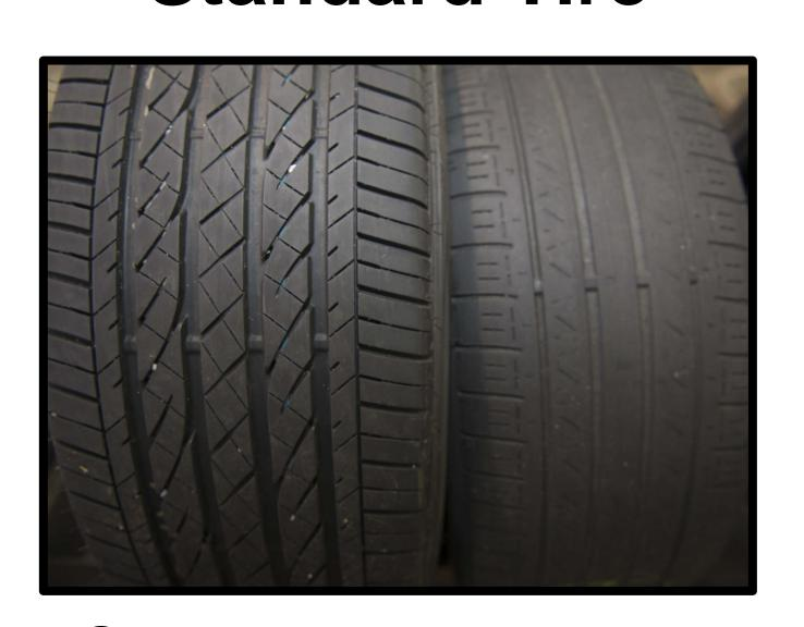
Snow tires have deeper grooves made to grip the snow for better traction.
