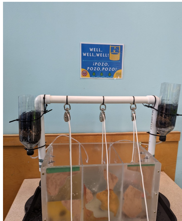
Figure 18 Improved Filtration System
