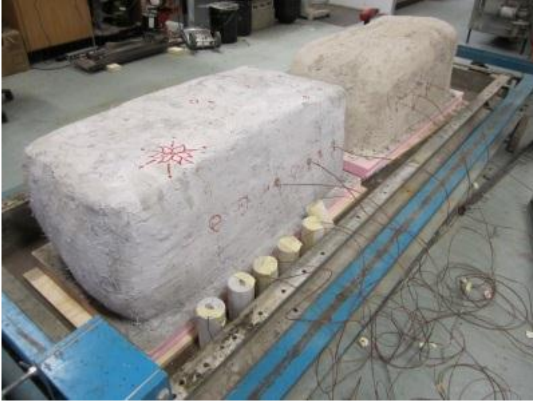
Figure 14: Specimens in Environmental Chamber for Thermal Resistivity Tests
