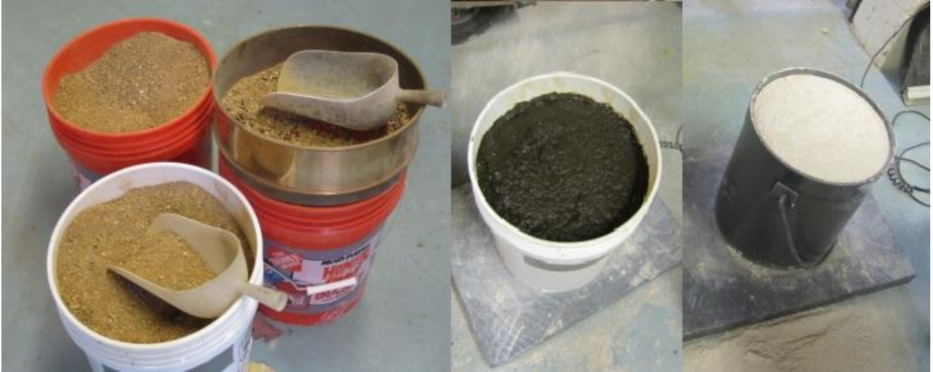
Figure 5: Sand, Manure, and Clay Used in Earthen Mixes
