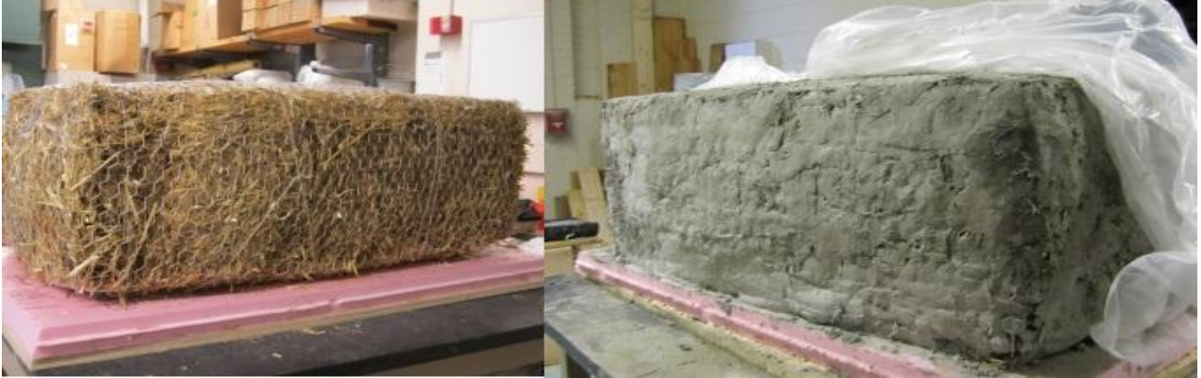
Figure 7: Pictures of CB Before and After First Plaster Coat Application
