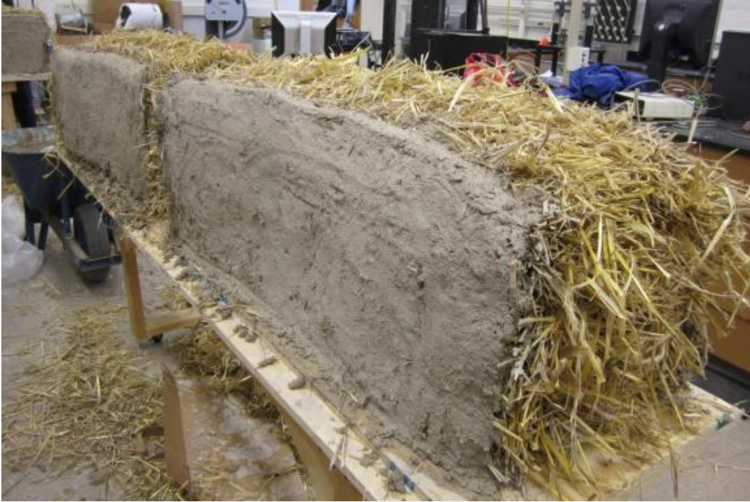
Figure 8: Dual-Sided, Earthen-Plastered Specimens After One Coat
