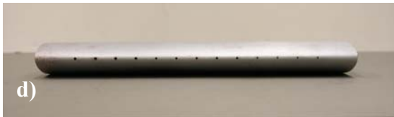
Figure 11: a) Dye injection system; b) dye valve connected to baseline foil; c) dye valve connected to 4L foil; d) leading edge of baseline foil with dye ports; e) leading edge of 4L foil with dye ports.
