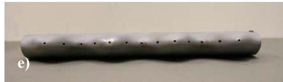
Figure 11: a) Dye injection system; b) dye valve connected to baseline foil; c) dye valve connected to 4L foil; d) leading edge of baseline foil with dye ports; e) leading edge of 4L foil with dye ports.
