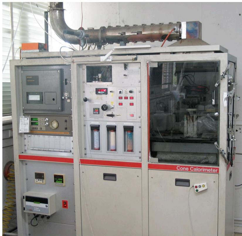
**Figure 6: Cone calorimeter at CSIRO**
