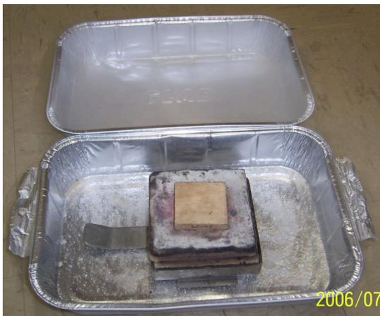
Figure 17: Liquid Nitrogen quenching apparatus
