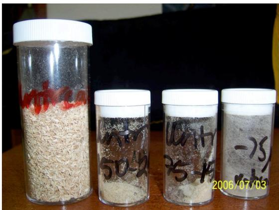
**Figure 21: Untreated Timber samples for TGA**
