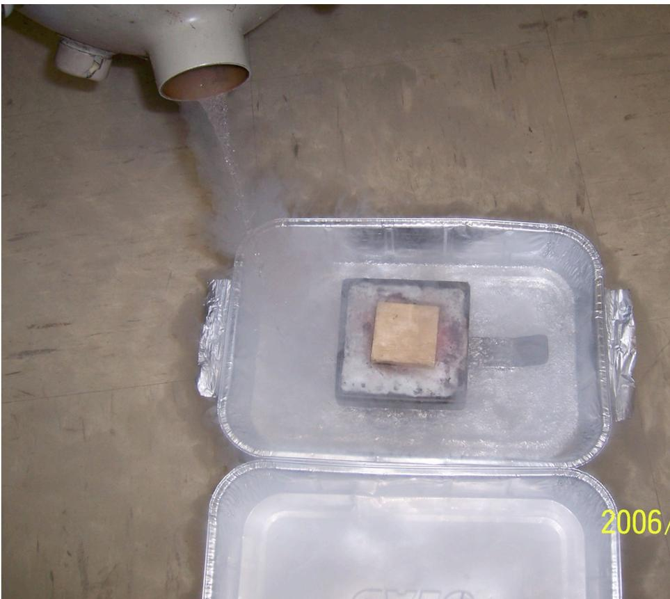
**Figure 18: Wood sample from cone being cooled**
