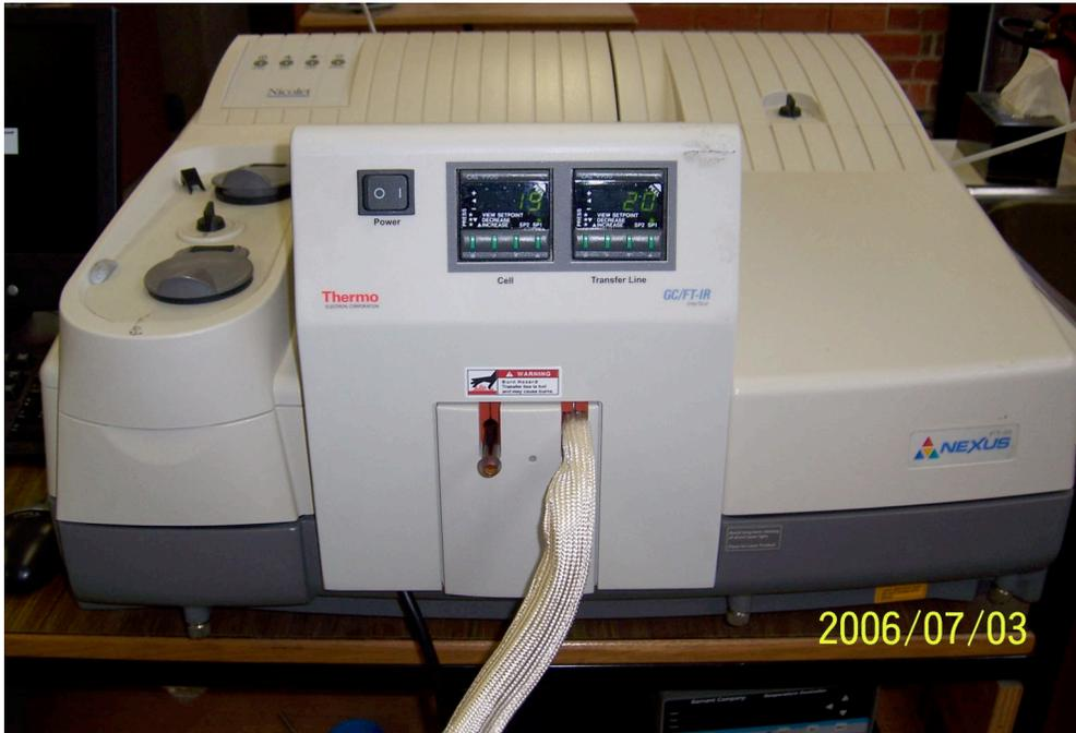
**Figure 9: FTIR Apparatus**
