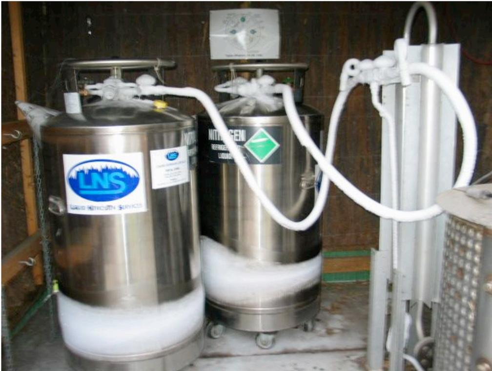
**Figure 20: Liquid nitrogen and glycol tanks**
