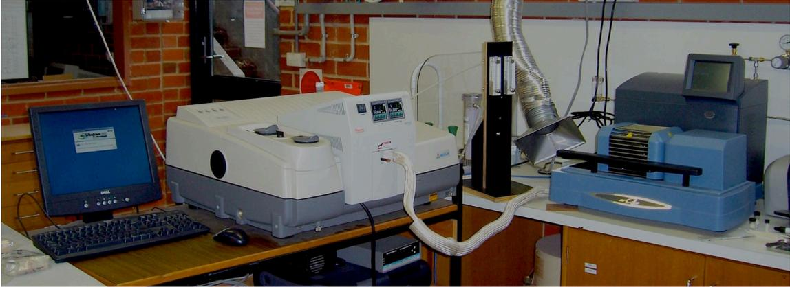
**Figure 10: FTIR and TGA-DSC equipment being used in conjunction**
