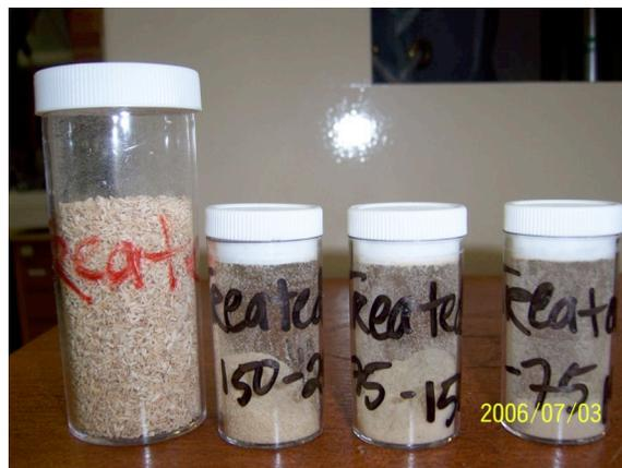
**Figure 22: Treated Timber samples for TGA**
