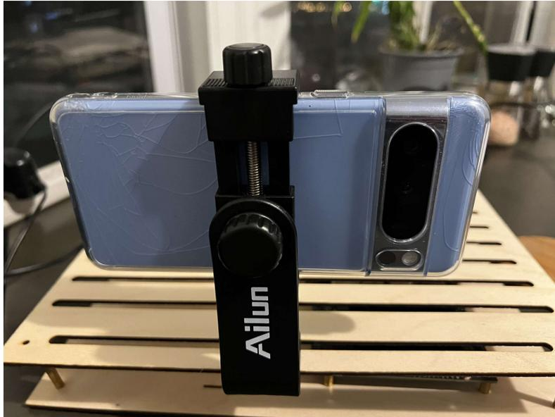
Figure 4.4: Picture of the Google Pixel 8 Pro attached to the capture rig.
