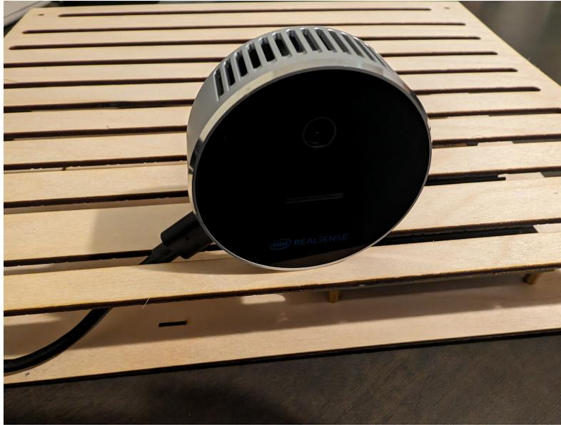
Figure 4.3: Picture of the Intel Realsense L515 Lidar camera attached to the capture rig.
