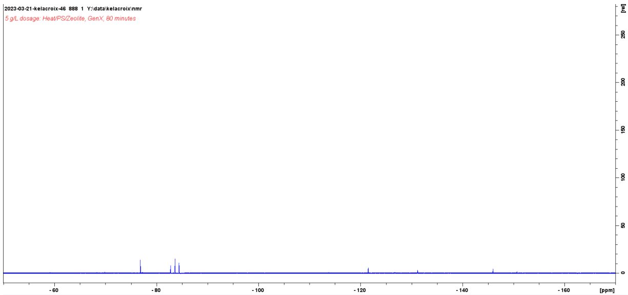
Figure 161. NMR Spectrum for the heat/PS/zeolite, PFOA reaction with 5 g/L dosage at 80 minutes
