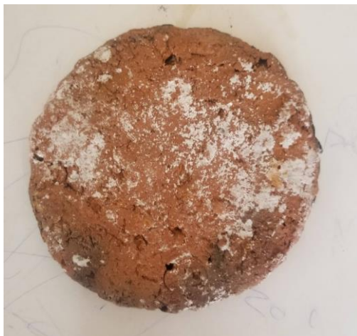
Figure 4: Clay-Sawdust Filter Made from 1:1 Ratio of Clay and Sawdust After Being Fired
