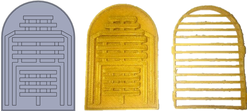
Figure 61 Mold design for the second iteration of the prototype (a) CAD model (b) FFF printed mold
