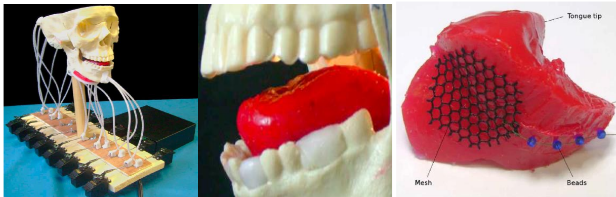
Figure 38 Anton animatronic model oral cavity view of actuating tongue (reproduced as is from [29]).
