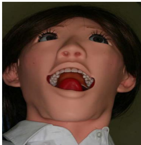
Figure 37 Dental robot front view of oral cavity with actuating tongue (reproduced as is from [28]).
