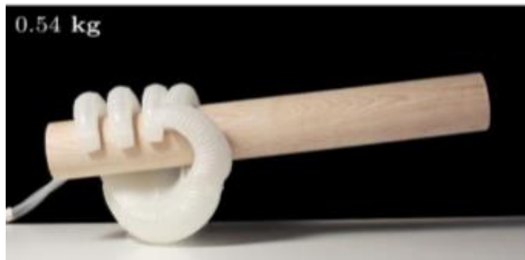
Figure 45 Underactuated robotic hand holding a rolling pin (reproduced as is from [37]).
