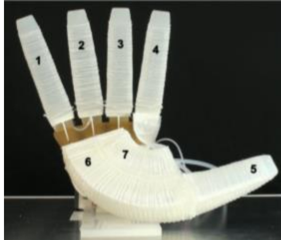
Figure 44 Underactuated robotic hand for dexterous grasping (reproduced as is from [37]).
