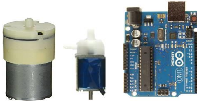
Figure 81 Major parts in testing control system (a) Miniature Air Pumps, (b) Solenoid Valves and (c) Arduino Uno Microcontroller.
