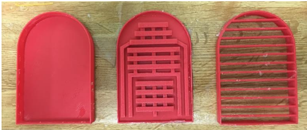
Figure 57 First tongue iteration 3D printed molds including (a) bottom layer, (b) top layer and (c) surface geometry layer.
