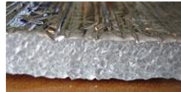
Figure 14: Prodex Total Insulation (Prodex, 2009)
