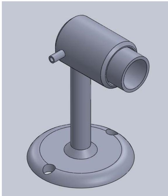
*Figure A-2. Cold cylinder and stand subassembly.*
