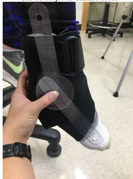
Figure 60: Goniometer Test – Plantar Flexion The test subject is Gillian Nadeau
