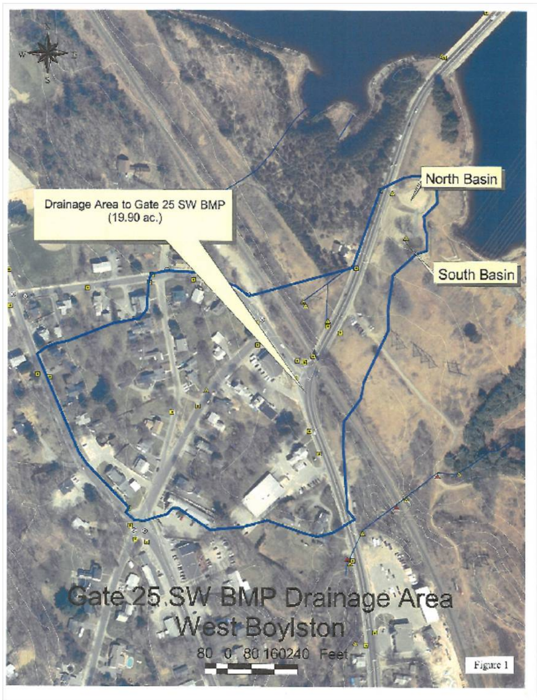
Figure 50: Drainage Area for Gate 25
