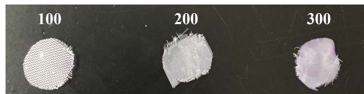
Figure 3: Nylon Mesh Discs. The discs were hole punched from sheets of 100, 200, and 300-gauge Ted Pella nylon mesh. Pore size decreases and mesh gauge increases from left to right.
