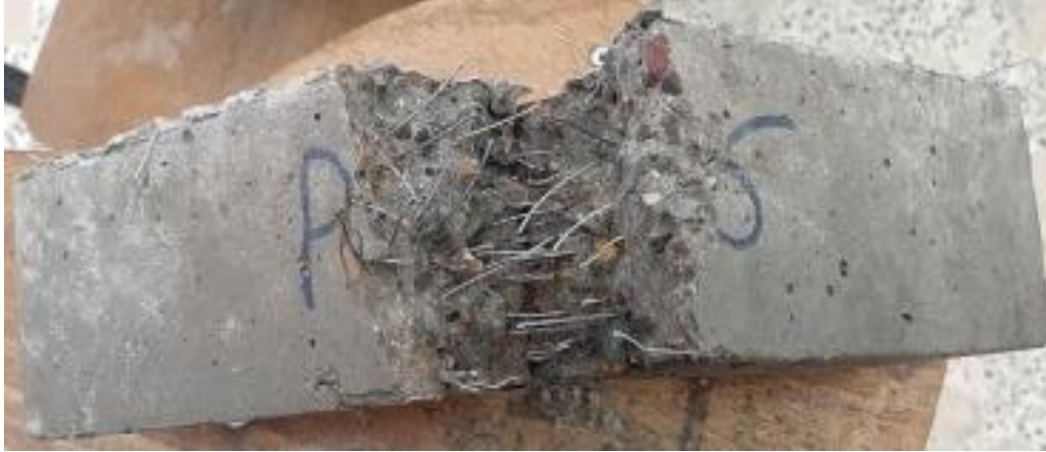
Figure 7: Representation of steel fiber inside of concrete
