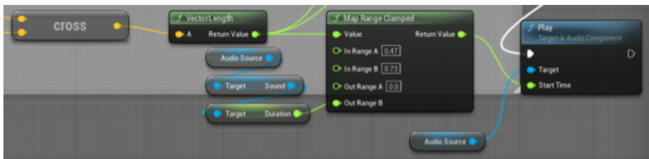
RecordPlayer Blueprint: using cross product to start song based off needle bone position.
