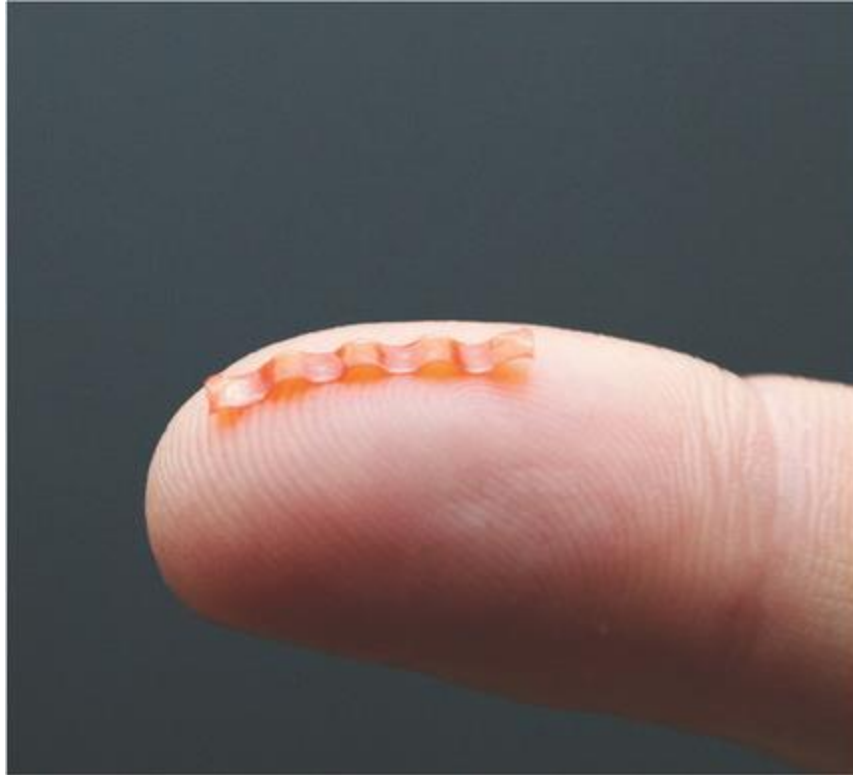
Figure 2.3 Soft Robotic Liquid Crystalline Elastomer Caterpillar from Light-Driven Soft Robot Mimics Caterpillar Locomotion in Natural Scale by Mikolaj Rogóż, et al.
