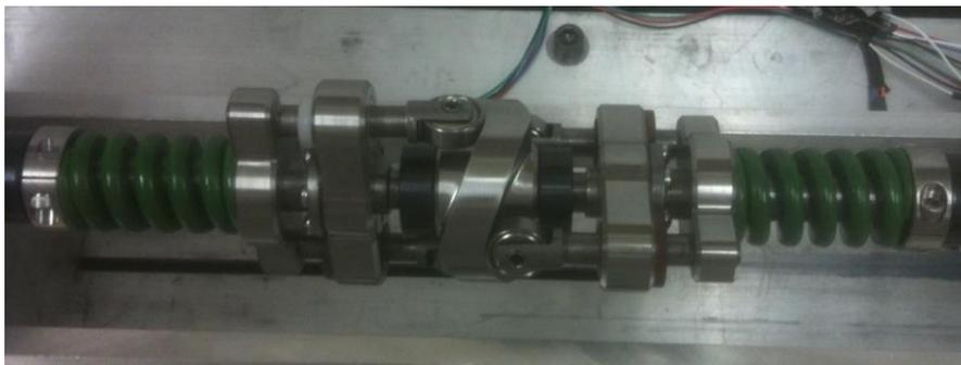
Figure 3 Collins et al's Cam Separation Spring (Collins, 2011)
