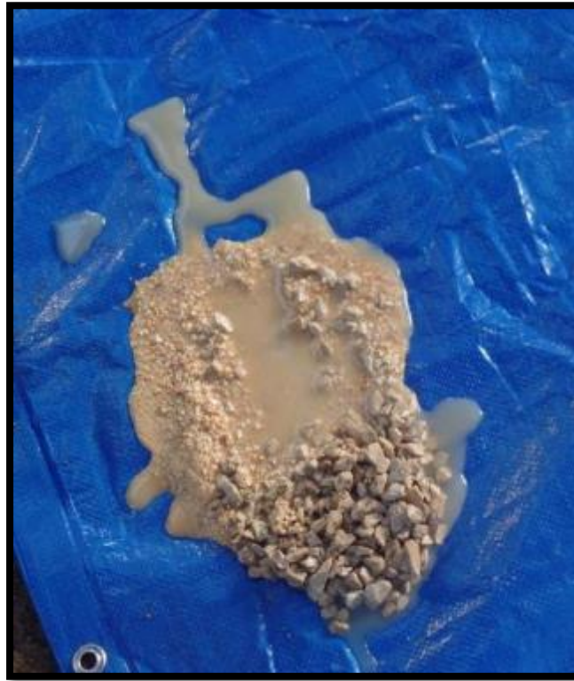
Figure 40. Remaining filter media from first trial mentioned above as the error in our attempt to backwash.
