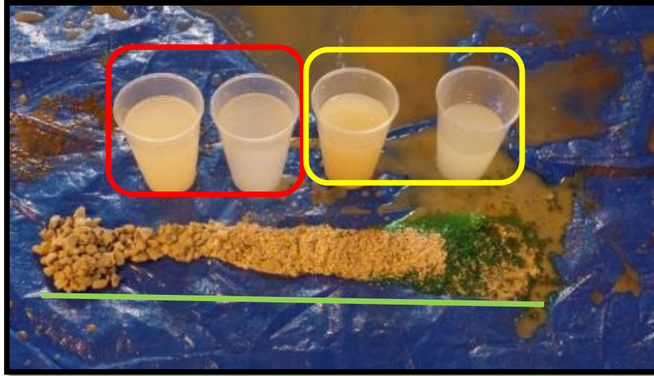
Figure 39. Results for glitter filtration Red rectangle represents the water out of the filter without contaminant added, yellow rectangles represent samples of water out of the filter after contaminant was added, green line underlines the filter media poured out after filtration and “backwash”.
