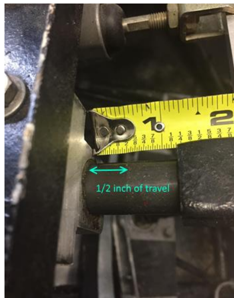
Figure 5: Measurement of Maximum Compression of the Hydraulic Brake Cylinders
