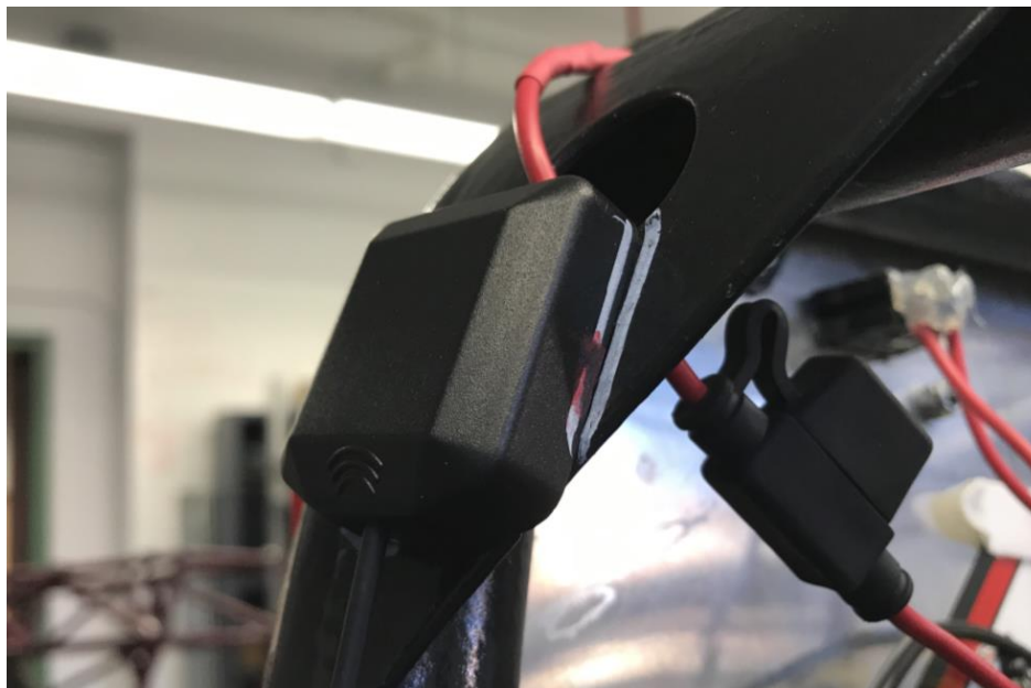
Figure 59. GPS Antenna Attached to Vehicle
