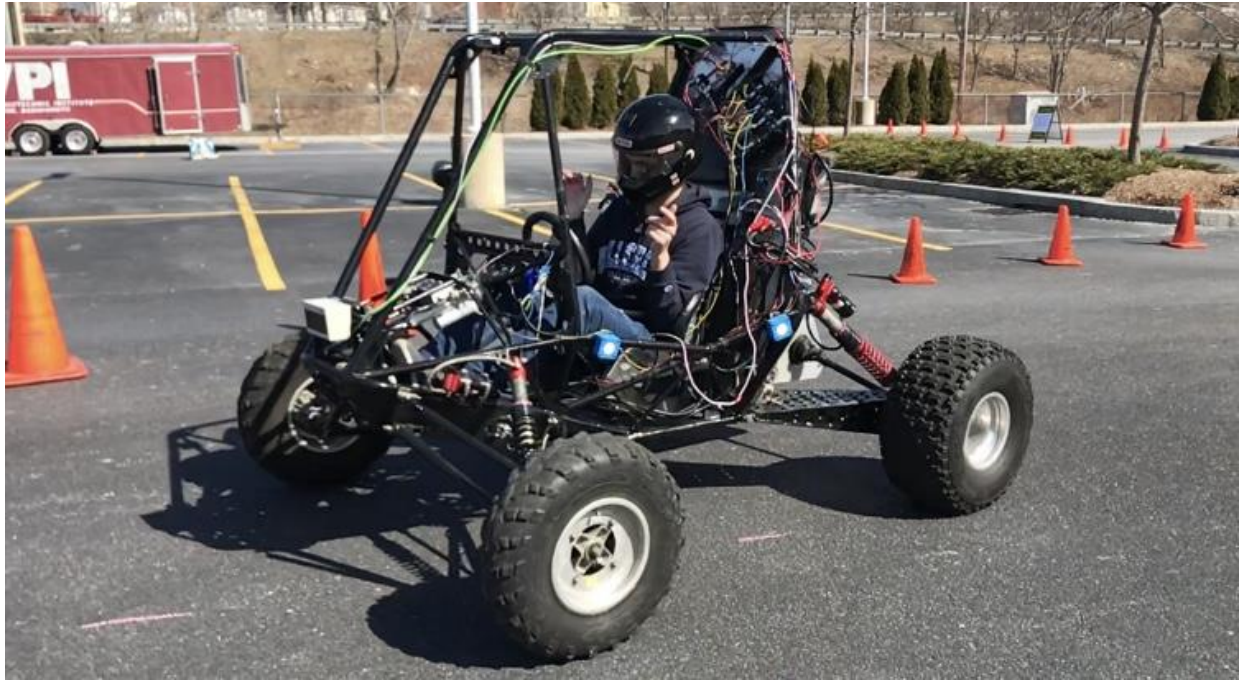
Figure 80. Baja Vehicle Traversing Parking Lot with No Human Intervention
