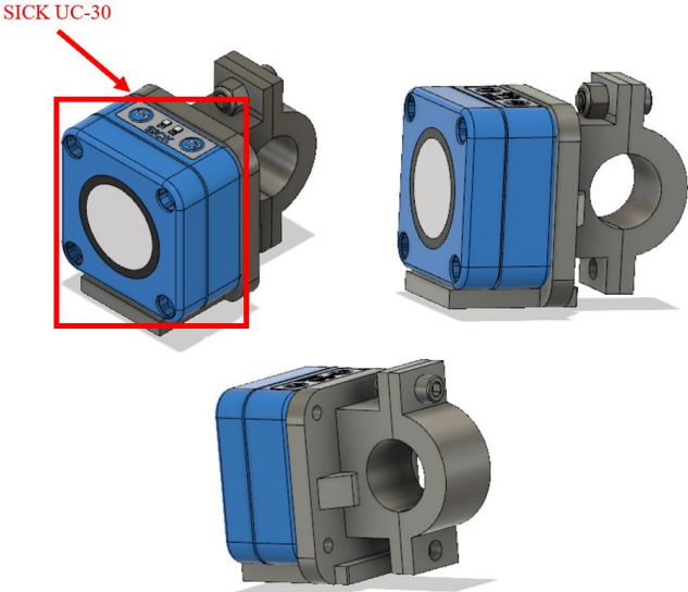
Figure 54. SICK Ultrasonics and Custom Side-Mount Model
