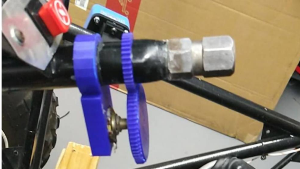
Figure 34. Potentiometer Cradle and Gears Printed and Mounted
