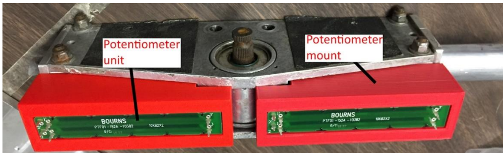
Figure 29. Top of Potentiometer Mount as Installed in Steering Rack
