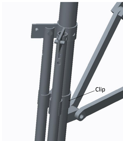
Figure 72: Support Legs in Locked in Cane/Crutch Position
