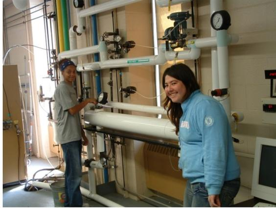
**Figure 1. Double Pipe Heat Exchanger Currently Used in the Unit Operations Laboratory.**
