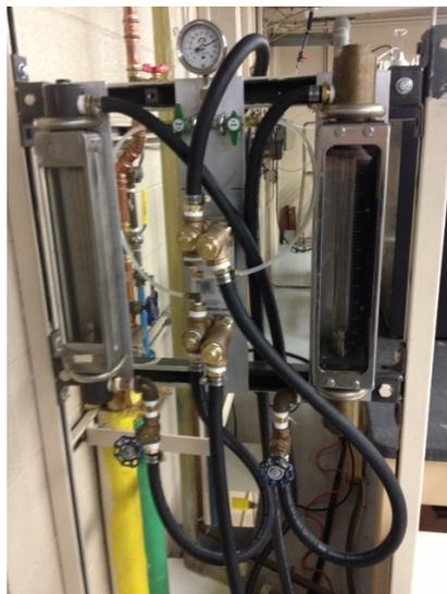
**Figure 2. Newly Installed Plate Heat Exchanger with Associated Hot and Cold Water Lines and Flow Meters.**
