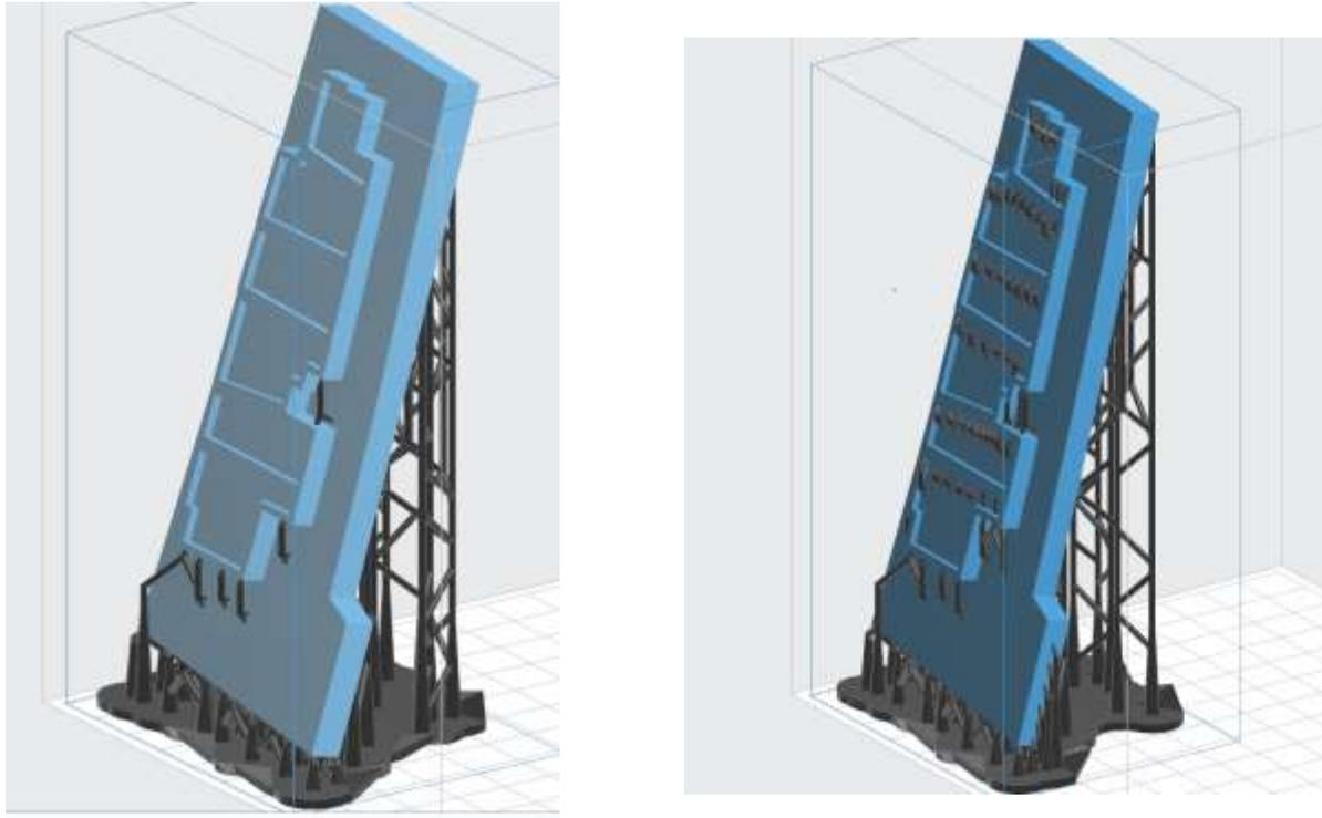
The model on the left is under-supported and will fail. The model on the right has more supports than it might need, but they are easy to remove and do not use up much resin. Once we started adding in extra support materials, our success rate started to increase.
