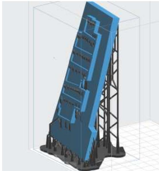
This method seemed to not be a good solution at first. The prints would still fail, but it appears that it was because the models were too large, not because the angle was too sharp. When 45 degrees was tried, both with a narrow side on the base and a wide side on the base, the failure rate was still high due to air pockets forming. Having a
