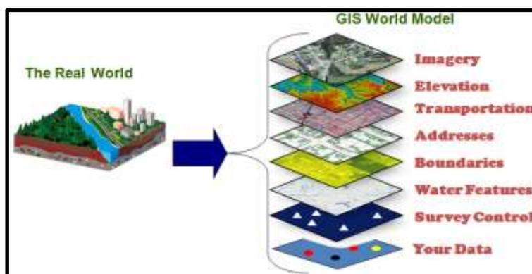
**Figure 9: Example of GIS Layers Commonly Used<sup>74</sup>**
