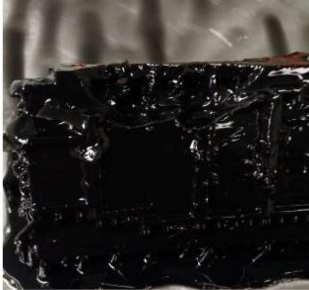
The print appears to have failed at one small point, which caused the failure to spread over a larger area as the more layers were added.
