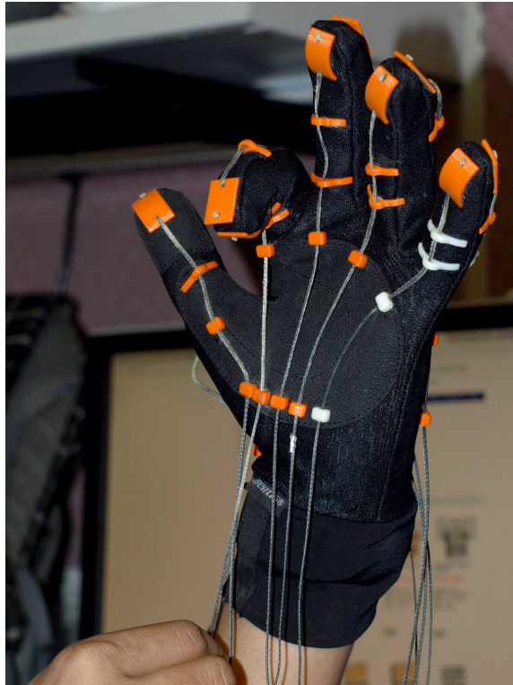
Figure 3.1: The soft tendon-actuated hand exoskeleton originally developed by Delph et al. [11]. 3D printed plastic cable guides (orange pieces) are attached to the palmar and dorsal surfaces of a neoprene glove. Kevlar cables are used as "tendons" to apply flexion and extension forces to the fingers.
