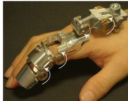
(c) In-line placement of IP joints with combined actuated rotation and sliding passive DoF at the MCP [101]
