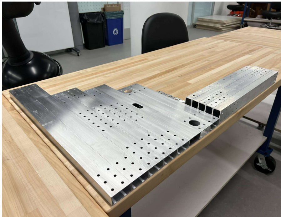
Figure 33 Chassis and payload storage structure components
