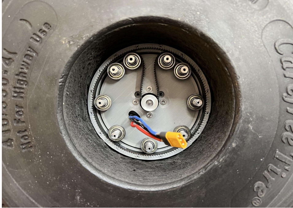
Figure 18 Hub inserted into the Carefree tire
