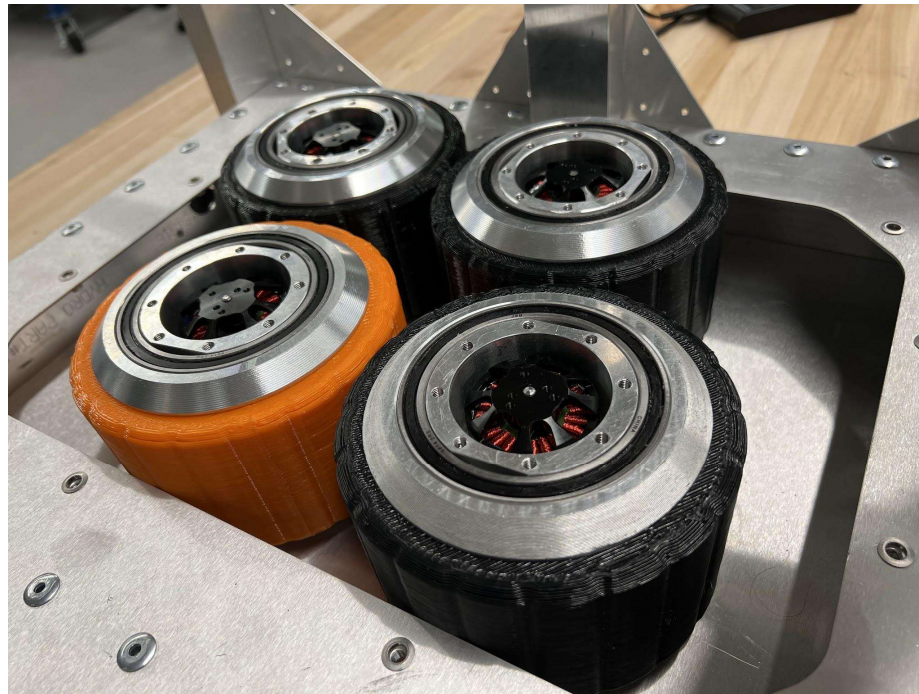
Figure 26 Fully assembled hub motors
