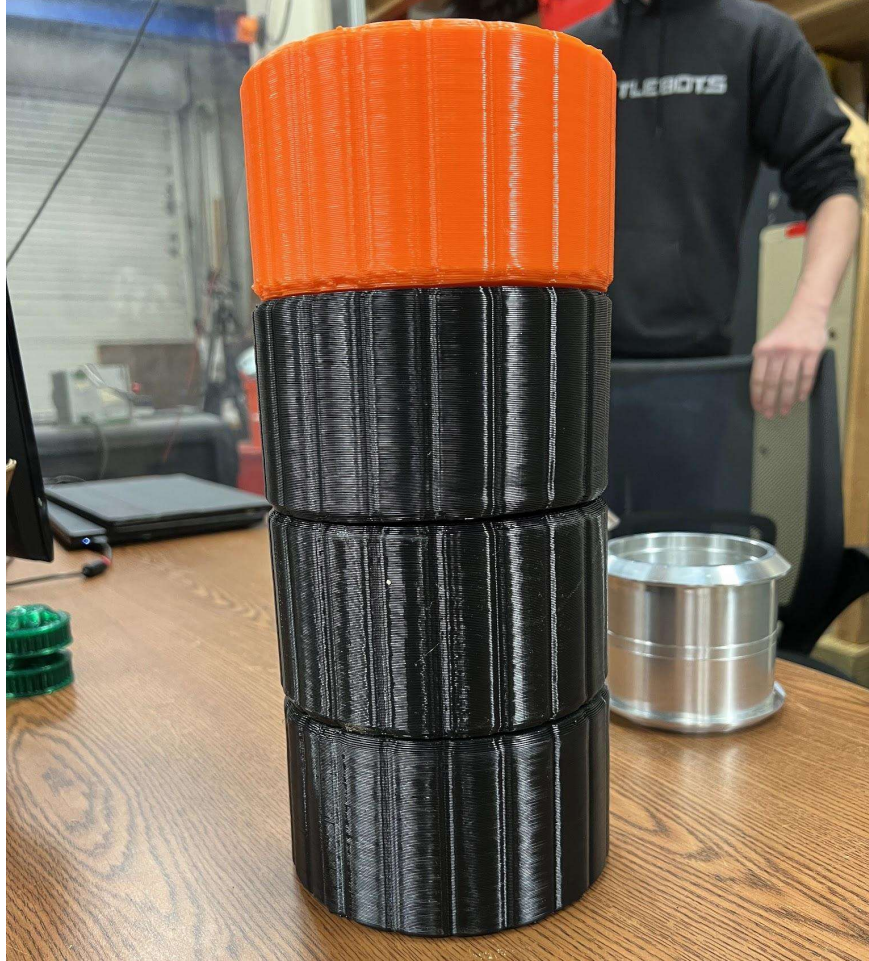
Figure 20 3D printed wheel hubs
