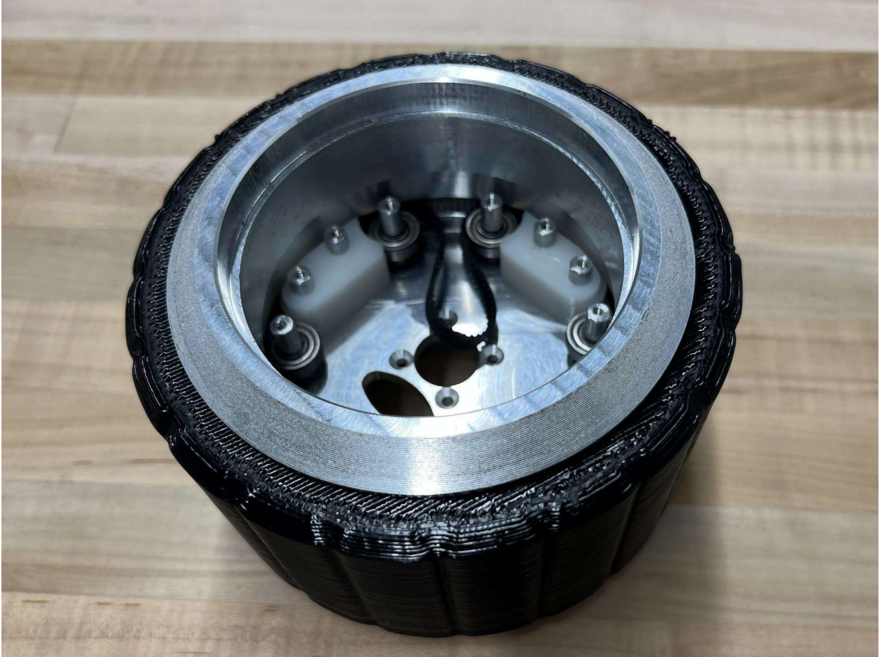
Figure 23 Split bearing and acetal retention system
