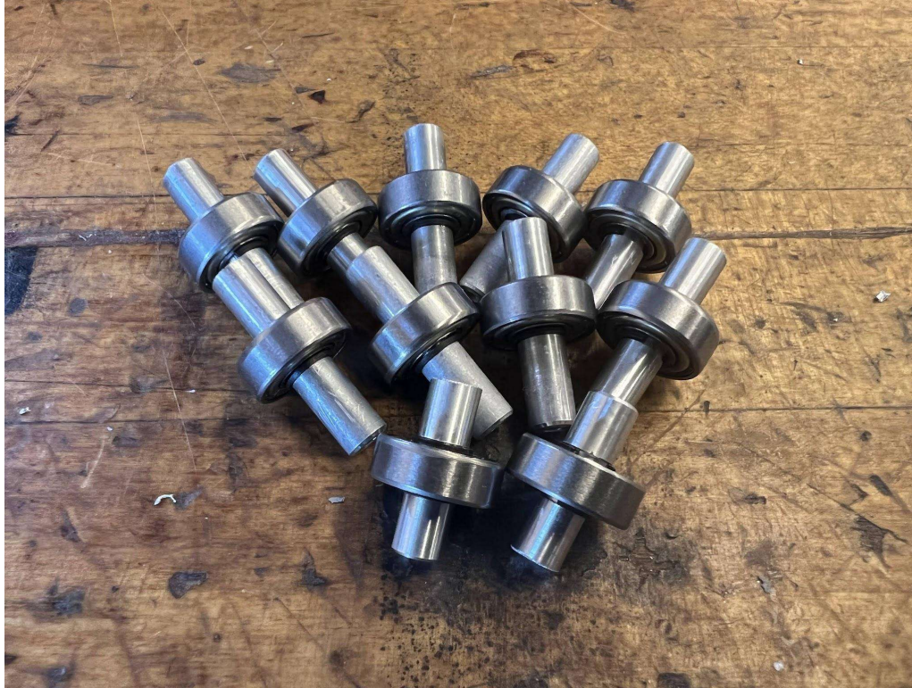
Figure 14 New Aluminum standoffs for bearing retention
