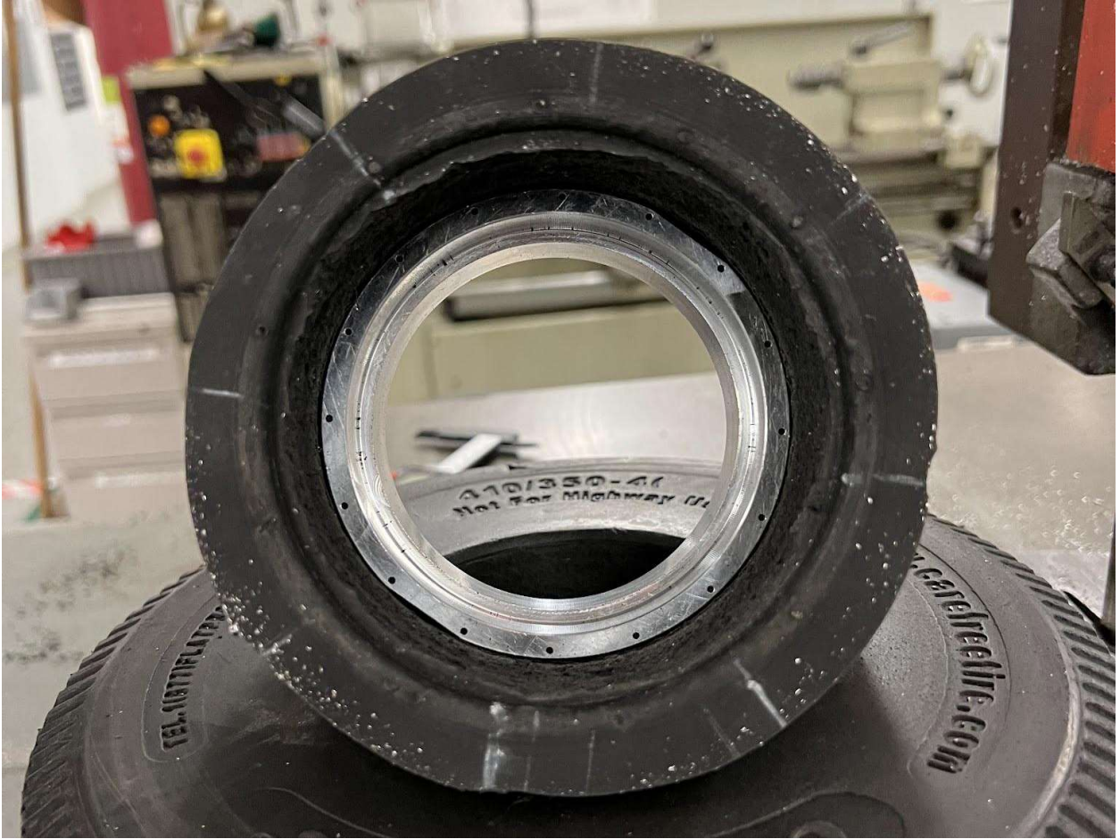
Figure 19 Attempted outer diameter reduction on a Carefree tire did not turn out concentric
