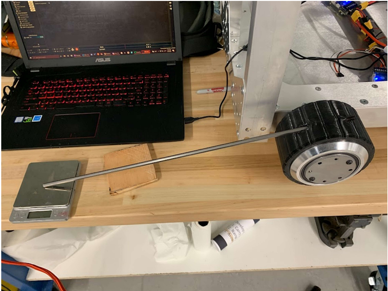
Figure 35 Startup torque testing of wheel assembly
