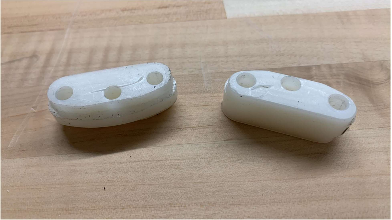
Figure 22 First version of acetal sliders
