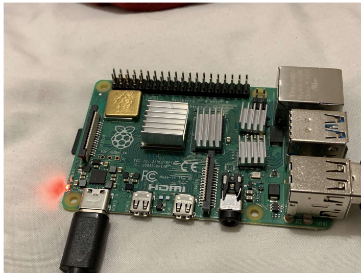
Figure 46 Raspberry Pi with heatsinks
