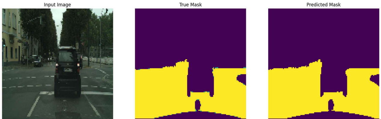
Figure 55 Comparison between input image, true mask, and predicted mask
