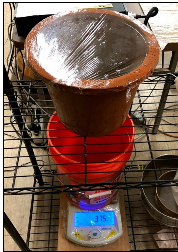
Figure 32: Single Filter Flow Rate Test
