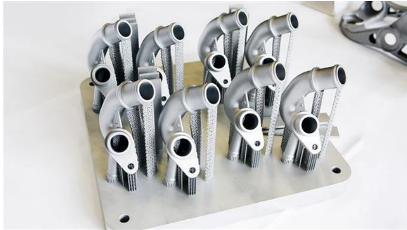
Figure 3: Water connector for Audi W12 Engine made by SLM Printer
