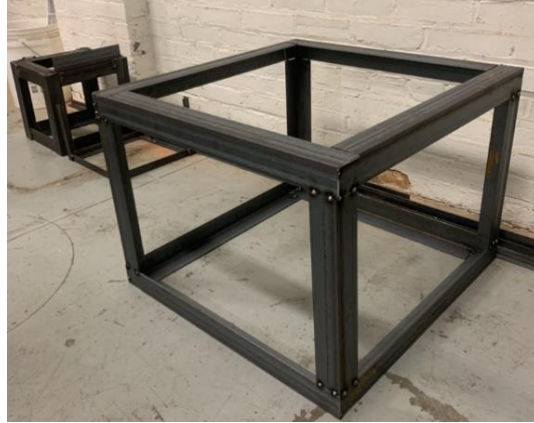
Figure 38: Welded chamber frames
