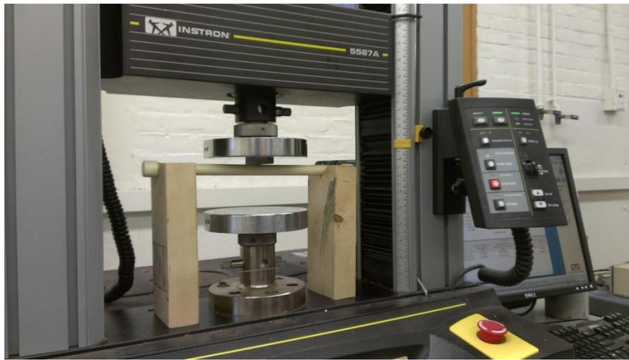
Figure 16: Image of Static Loading on Prototype 1.0 Series (Photo Taken by David Magnano)
