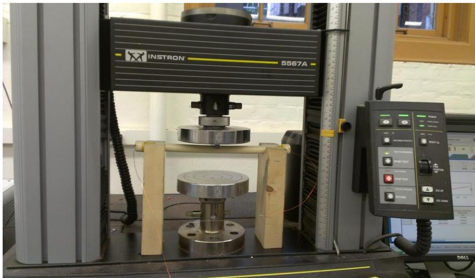
Figure 33: Image of Static Loading Test Performed on WPI's Instron 5567A (Photo Taken by David Magnano)
