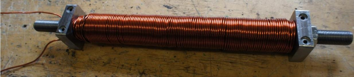
Figure 73: Picture of Prototype 3.0 Core and Magnetic Coil (Photo Taken by David Magnano)
