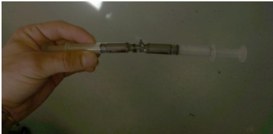
**Figure 21: MR Fluid Sample in Connected Syringes (Photo Taken by David Magnano)**
