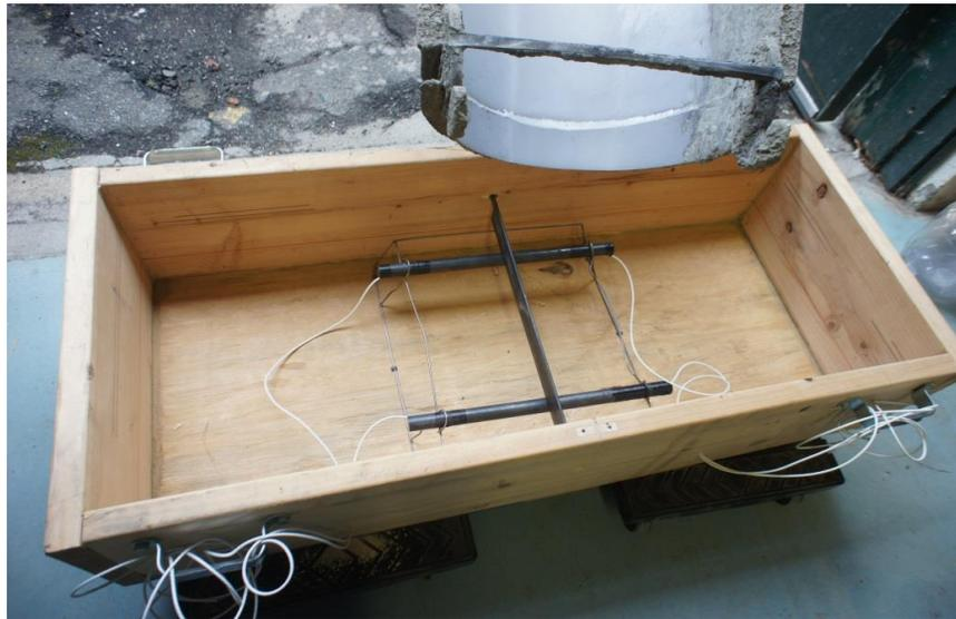
Figure 9: Empty Slab Mold with Dowels place on chairs with strain gages attached (Photo Taken by David Magnano)
