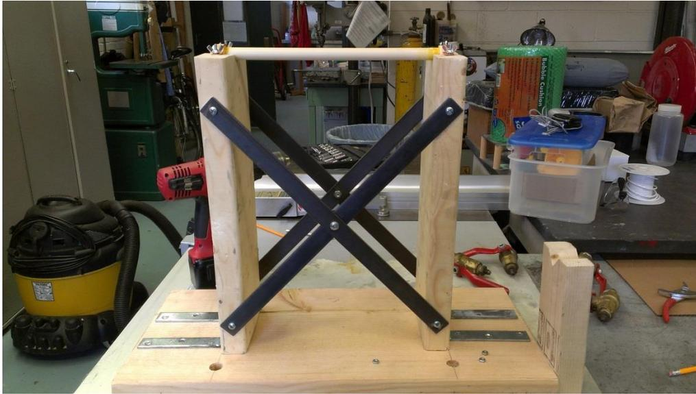
Figure 18: Testing Apparatus for Impact Loading (Photo Taken by David Magnano)
