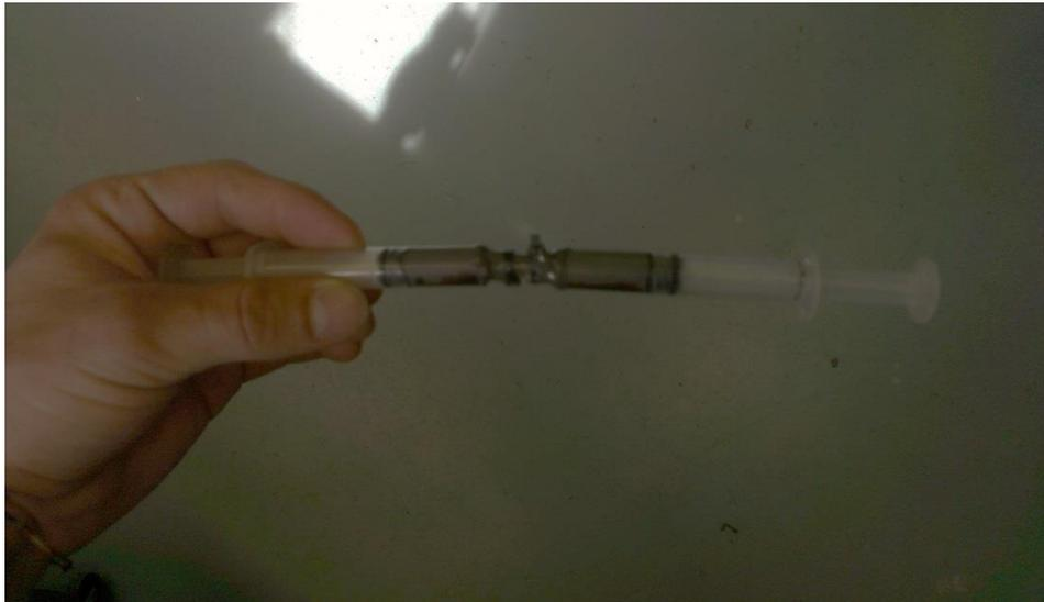
Figure 59: MR Fluid Sample in Connected Syringes (Photo Taken by David Magnano)
