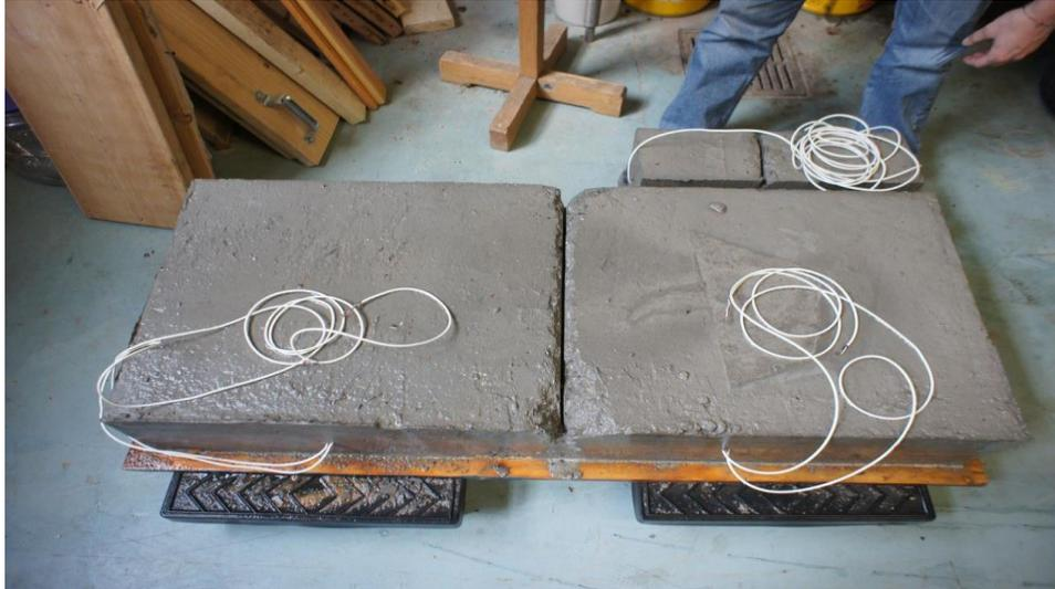
Figure 10: Slab After Curing with strain wires attached to the dowel protruding from the concrete
