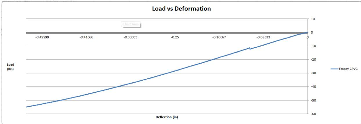
Figure 26: Test 1, Empty CPVC Deflected to .5"
