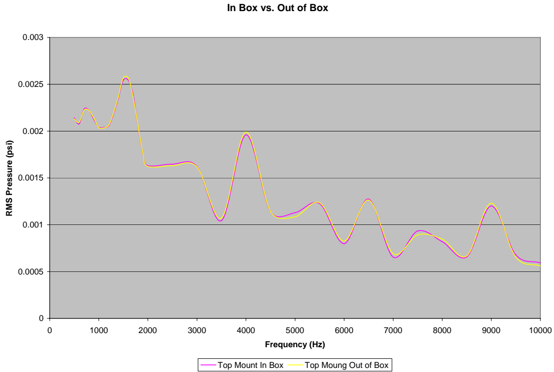
Figure 25 - In Box vs. Out Box Pressures
