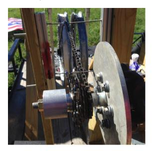
Figure 23: New Gear Train
