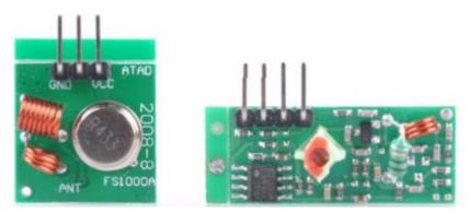
Figure 10: UCEC XY-MK-5V / XY-FST 433Mhz RF Transmitter and Receiver Link Kit
