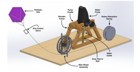
Figure 29: Complete CAD assembly of kite power system (excluding chain tensioner and kite wheel supports)
