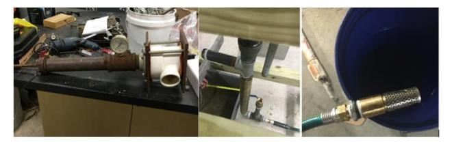
Figure 30: Old pressure valve (left) versus new surface pumping system (center, right).
