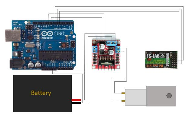
Figure 12: Circuit Diagram of Motor Configuration
