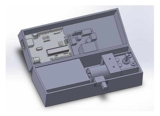
Figure 14: Initial CAD of circuit organization in casing
