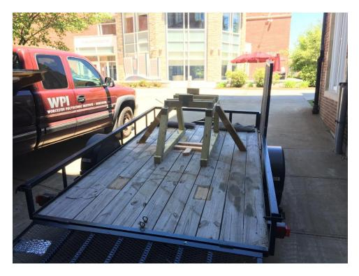
Figure 37: Frame secured to trailer with added 45-degree supports
