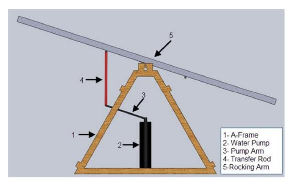
Figure 7: SolidWorks Model of Rocking Arm Design (Bartosik et al. 2012)
