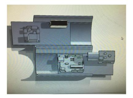
Figure 13: Initial CAD of circuit organization in casing
