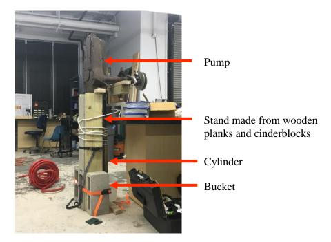
Figure 26: Reduced pump subsystem test setup
