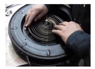
Figure 18: Inside a Linear Reel Spring
