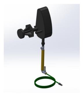
Figure 32: Full pump assembly including surface pumping
