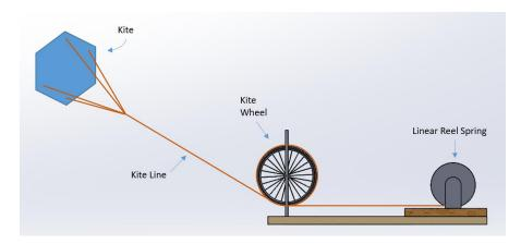
Figure 20: Kite Line Torque Transfer Method
