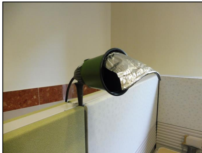
Figure 33: Small Aluminum Shield and Plastic Flower Pot added to the Circular Spotlight
