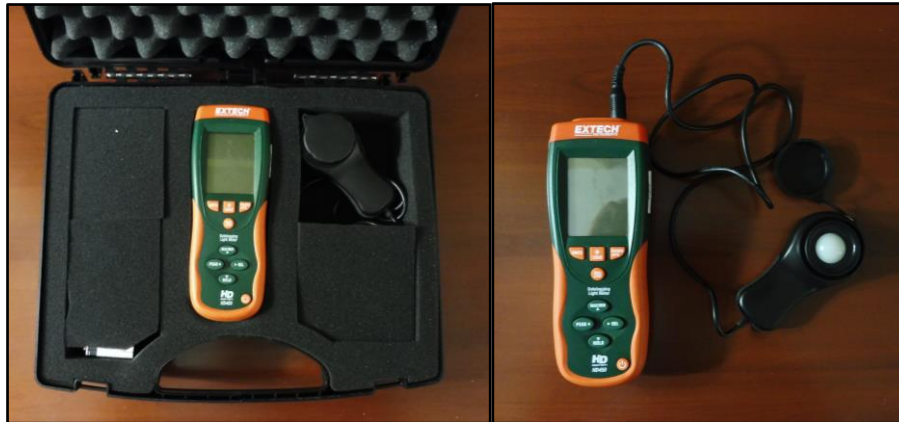
Figure 26: Unassembled Photometer in the Carrying Case and Assembled Photometer
