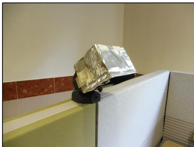
Figure 30: Two Shields Added to the Square Flood Light
