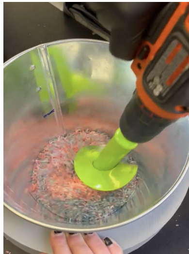
Figure 20: Mixing test of green auger attachment
