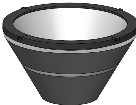
Figure 51: Final compost chamber subassembly
