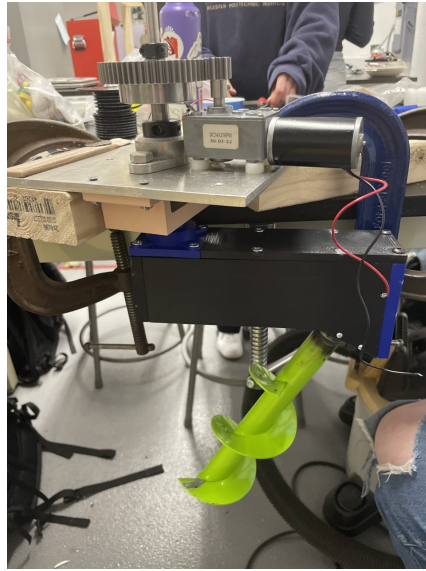
Figure 44: Fully assembled orbital mixing arm
