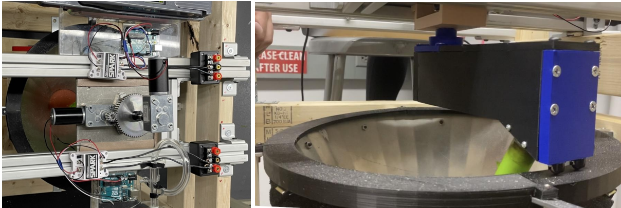
Figure 45: Setup for secondary testing of the mixing system transmission
