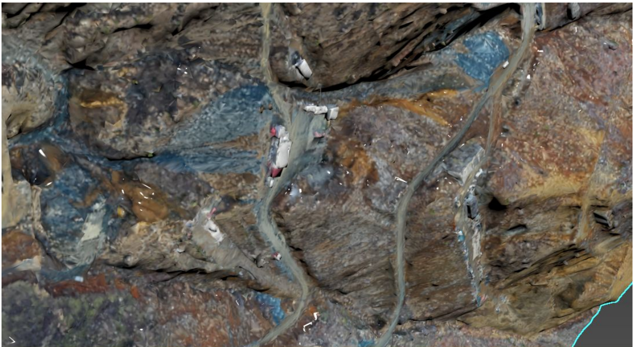
Figure 14: A portion of the terrain model after being compressed to 20% the original vertex amount.
