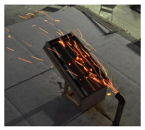
*Figure 1: The NIST Dragoon firebrand shower at 6 m/s attacking concrete roof tiles in a test conducted to show how firebrands slip under roofing tiles* [a]
