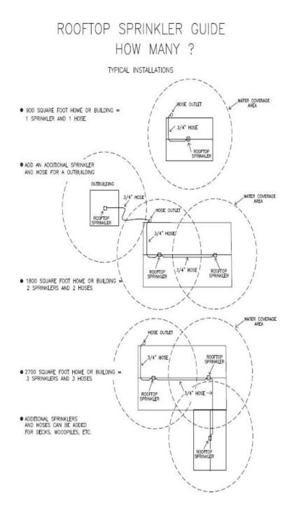
Figure 9: RoofSaver Sprinkler and Roof Installation Guide [m]
