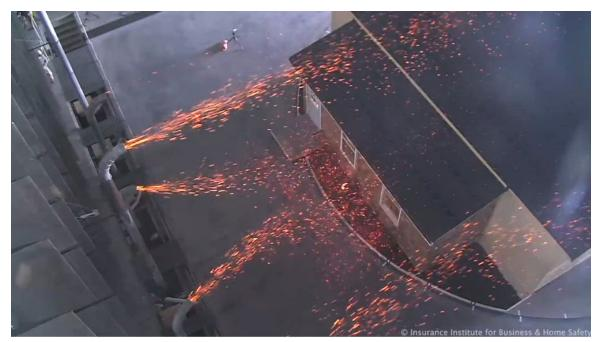
*Figure 2: A 2013 IBHS test with firebrand ember generators to simulate a UWI wind storm igniting a residential building* [b].
