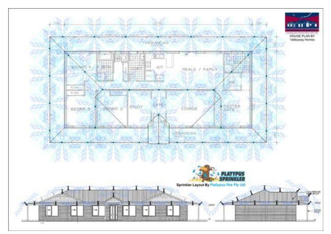
Figure 11: Example Platypus installation diagram showing the areas of coverage, sprinkler locations, piping arrangements, and layout for a roof Size of 12 x 24.6 meters [n].
