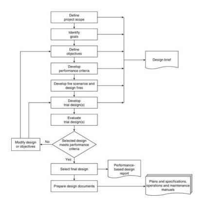
Figure 12: SFPE Performance-based design flowsheet used to frame the system standard [o].
