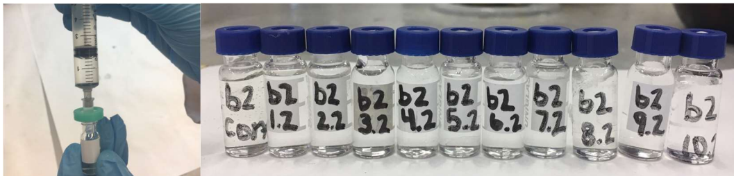
Figure 13. Photograph on the left is an example of moving the effluents into the 2mL vial with the aid of a nylon filter. The left image shows all the collected effluent for the second trial of Blak I biochar. Both photographs were taken in the BIOTAR lab.
