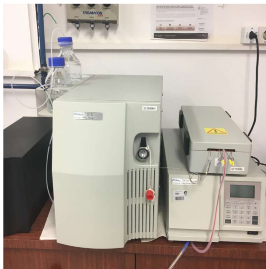
Figure 16. Photograph of HPLC unit used to determine the concentration of sugar in the effluent. The picture was taken in the BIOTAR lab.
