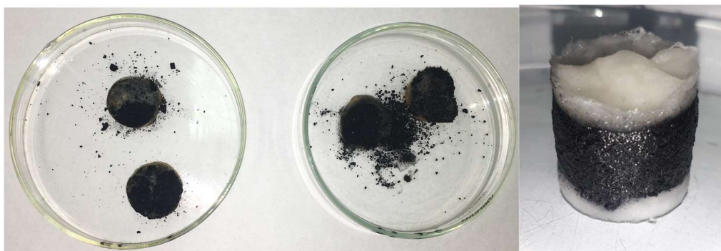
Figure 14. The photograph on the left is of activated carbon after it was removed from the column and dried in the oven. The image on the left is biochar after it was removed from the column. Both photographs were taken in the BIOTAR lab.
