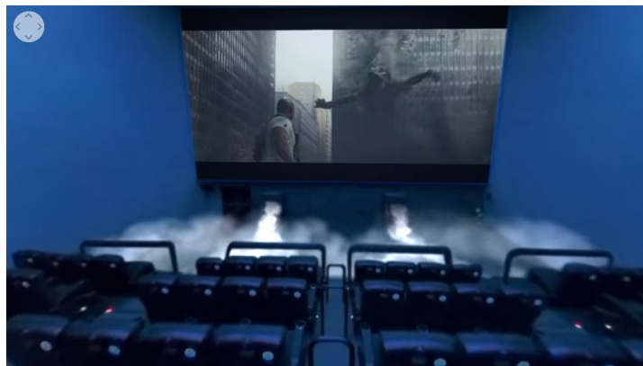
Figure 68. Smoke machines installed inside the seats and in front of the projection screen create a mist while the seats, controlled automatically, can also move at a fixed angle.
