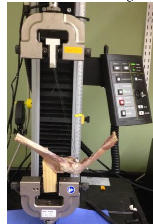
Figure 3: Test set-up for t translation clinical assessment simulation
