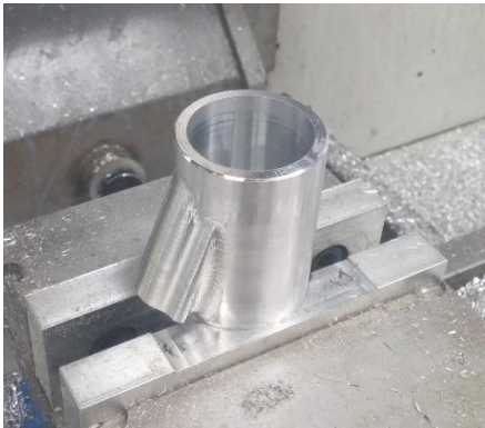
Figure 118: Intake runner operation 3
