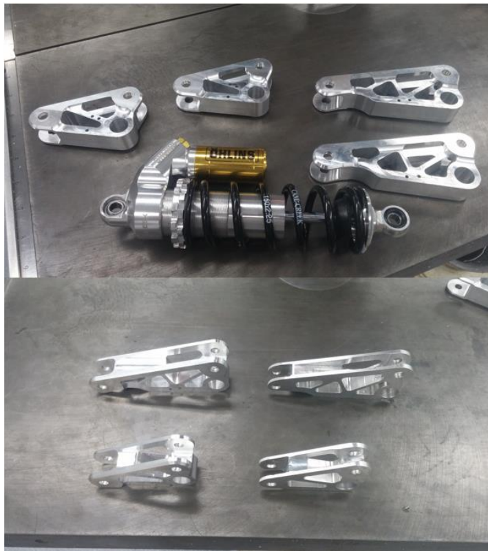
Figure 51: Upper: Manufactured Revision 2 Rockers; Lower: Revision 1 & 2 Rocker Comparison
