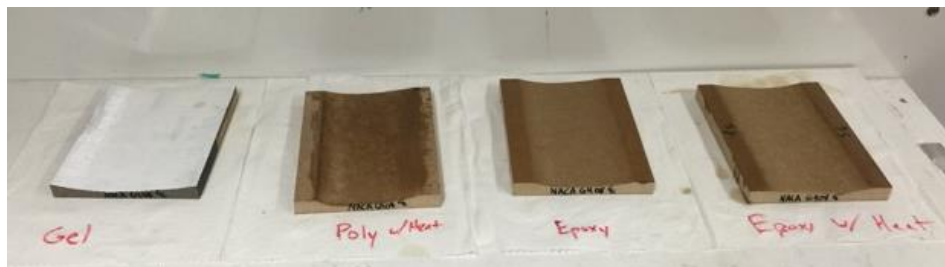
Figure 150: Mold Sealing Test
