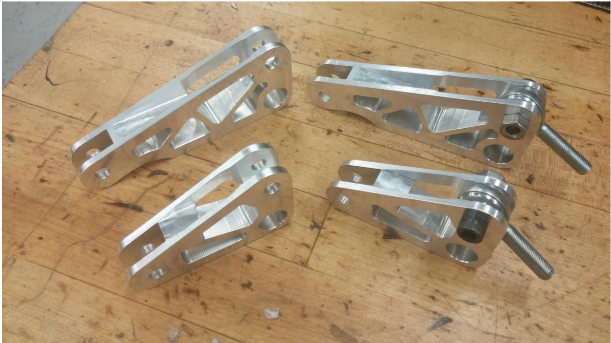
Figure 47: Machined Revision 1 Rockers
