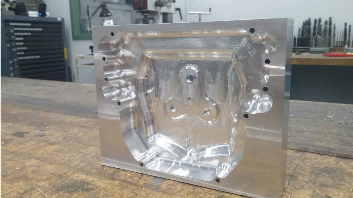
Figure 106: Finished Internal Section of the Back of the Steering Wheel
