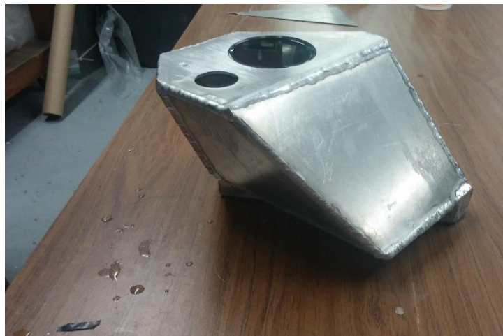
Figure 113: Checking fuel tank for leaks
