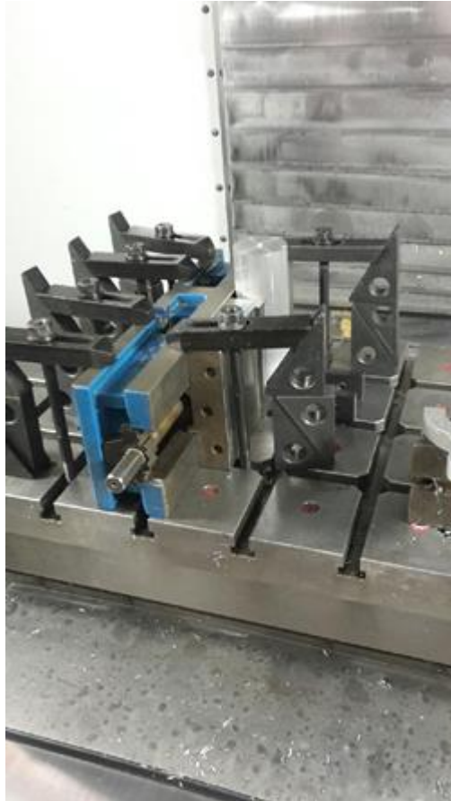
Figure 122: Fixturing for Mill op of Restrictor
