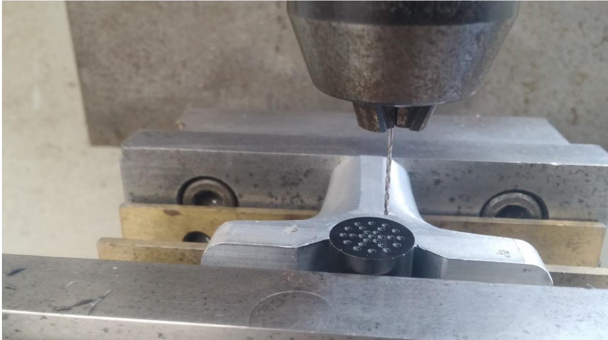
Figure 108: Pogo Pin Connector Drilling Operation
