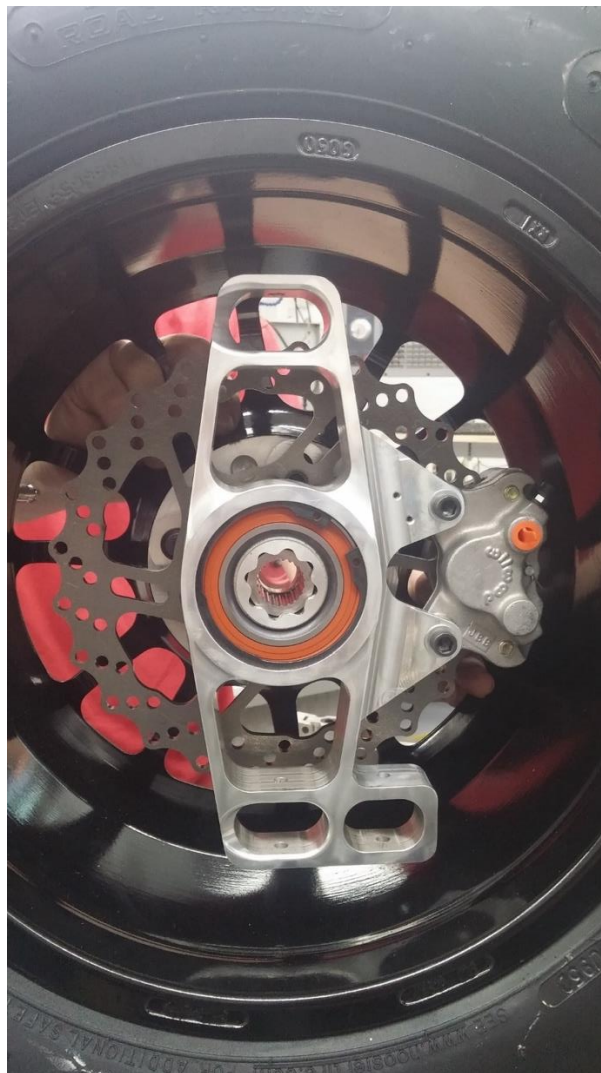
Figure 138: Rear hub spline design with steel spline insert installed
