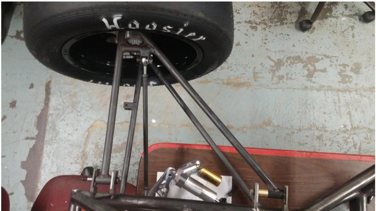
Figure 30: Basic rocker layout [Rear]
