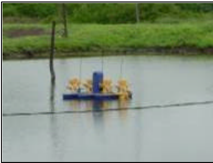
Figure 3-3 Example of a floating aerator.
