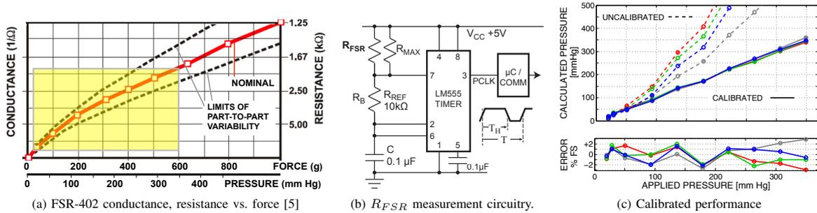
Fig. 3. Measurement technique for resistive force sensor.
