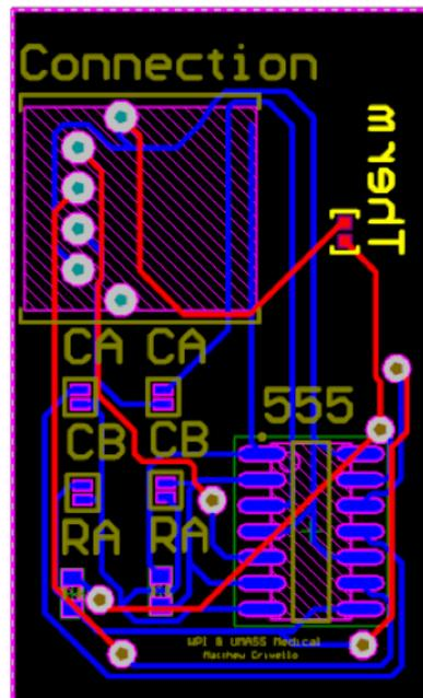
FIGURE E.2: Electrical Prototype PCB (net routes)
