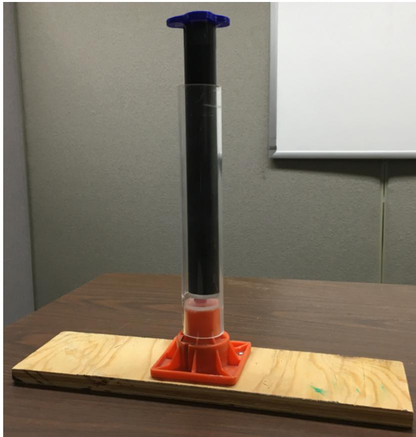
FIGURE 3.9: Force Sensor Calibration Apparatus
