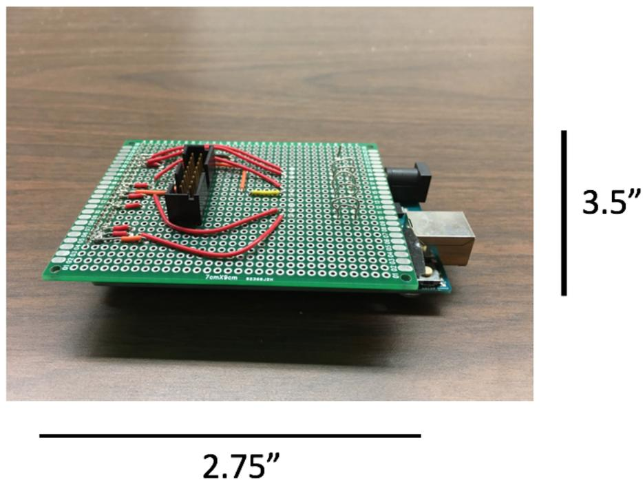
FIGURE 3.12: Arduino Mega Board with Mezzanine Board
