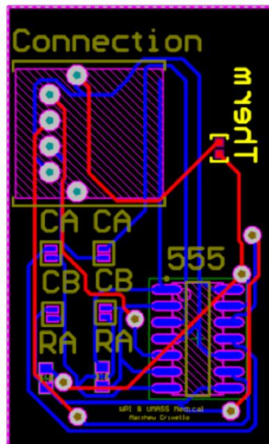
FIGURE 3.4: Electrical Prototype PCB (net routes)
