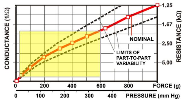
Fig. 1. Conductance vs. force for FSR-402 sensor [4].
