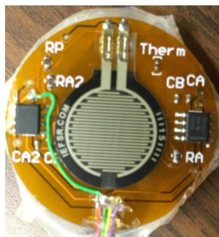
FIGURE 3.16: Completed Flex PCB Prototype with Modification
