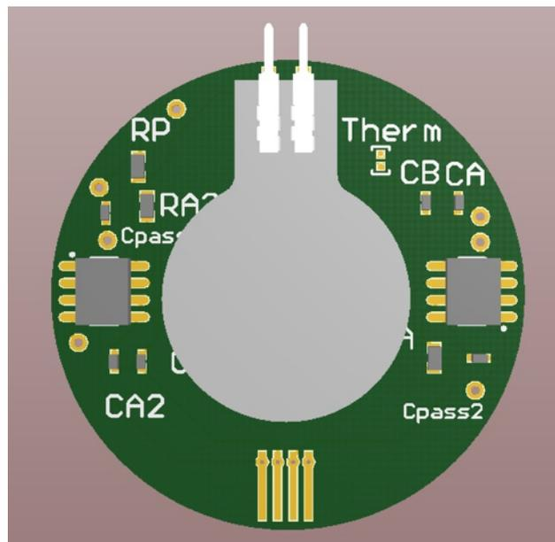
FIGURE F.3: Flex PCB Prototype 3D Rendering
