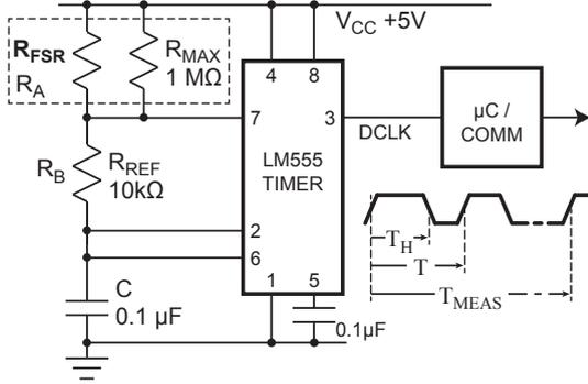
Fig. 2. System block diagram with time-based resistance measurement.
