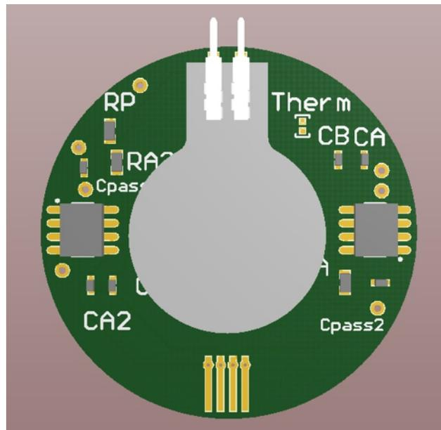
FIGURE 3.14: Flex PCB Prototype 3D Rendering
