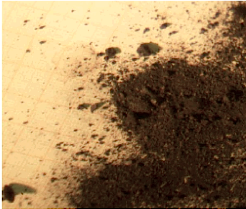
Fig. 2.2 Above: Dust from a failed fuel rod on a 1 cm grid (13, NRC NUREG)
