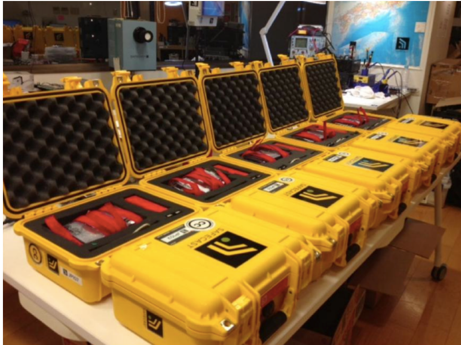
Fig. 2.4 Above: GPS-enabled, networked bGeigie test gear, (27, Safecast)
