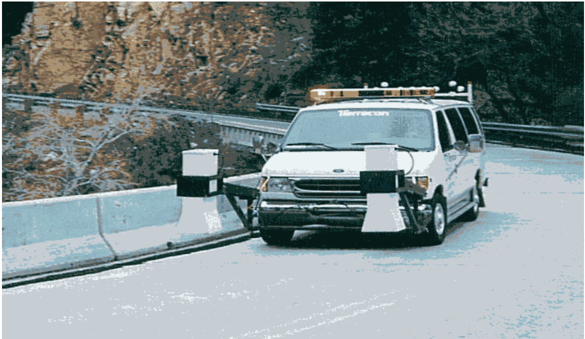
Figure 14. Photo of Ground Penetrating Radar System. Courtesy of Infrasense, Inc. web page.
