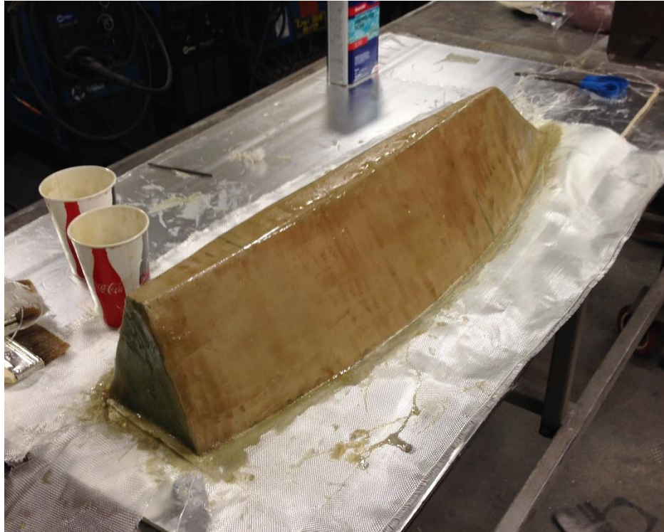
Figure 36: Vaka hull after application of fiberglass cloth and resin.
