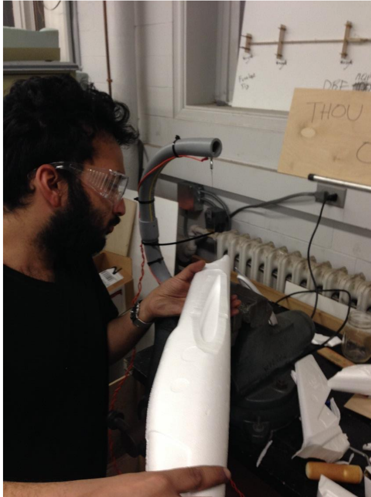
Figure 37: Foam fuselage being cut with a hot wire foam cutter.
