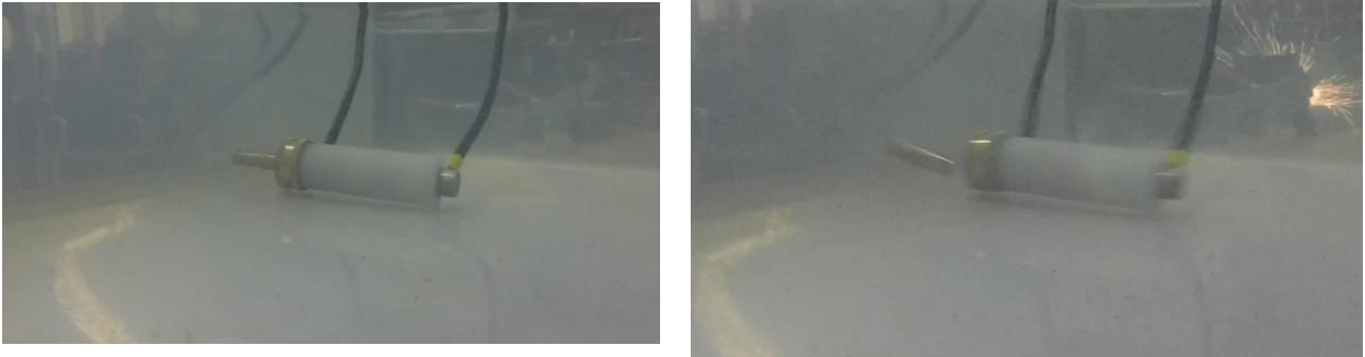
Figure 23: Still frames from chamber 4 underwater test during which the nozzle broke.
