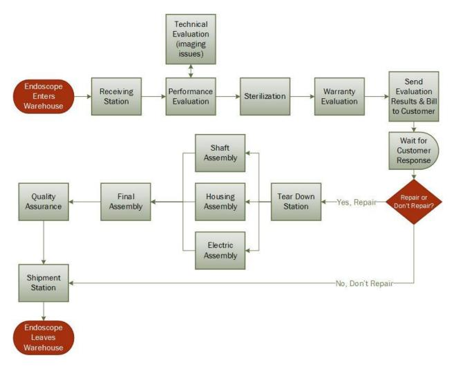
Figure 8: Current repair process map for returned Legacy Gastroscope at KARL STORZ's Charlton, MA facility.
