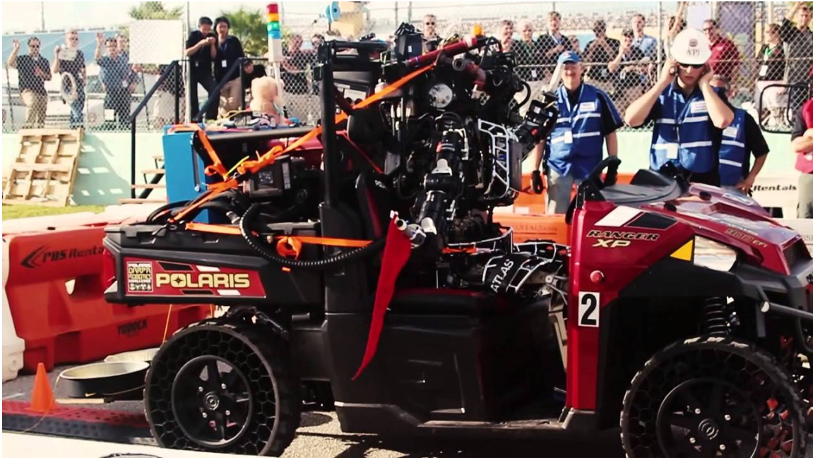
Figure 10 - In this shot, an ATLAS belonging to Worcester Polytechnic Institute begins the driving task. Source: DARPA
