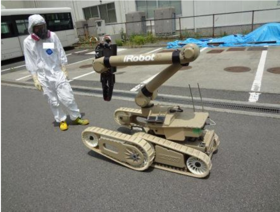
Figure 16 – An iRobot Warrior, used for hazardous waste clean-up, search-and-rescue, and explosive ordnance disposal missions in Iraq and Afghanistan, drives across the grounds of Fukushima-Daiichi. Warrior is one of several robots that wasn't quite up to the challenge of saving Fukushima. Source: Tokyo Electric Power Company.
