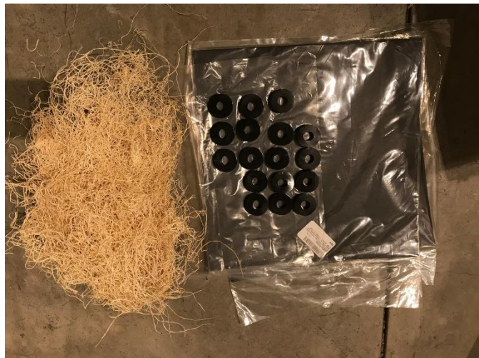
Figure 10 - Excelsior (left), Sorbothane (disks in center), and PORON (right rectangular padding)
