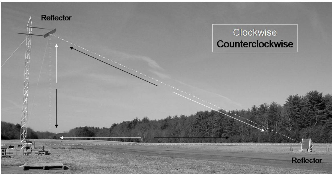
Figure 3.1 – Image of equipment setup showing direction of signal transmission
